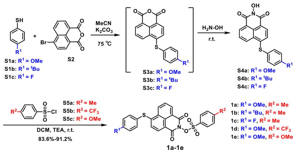
Scheme 1 Synthesis of nonionic sulfonate ester PAGs **1a–1e**.
