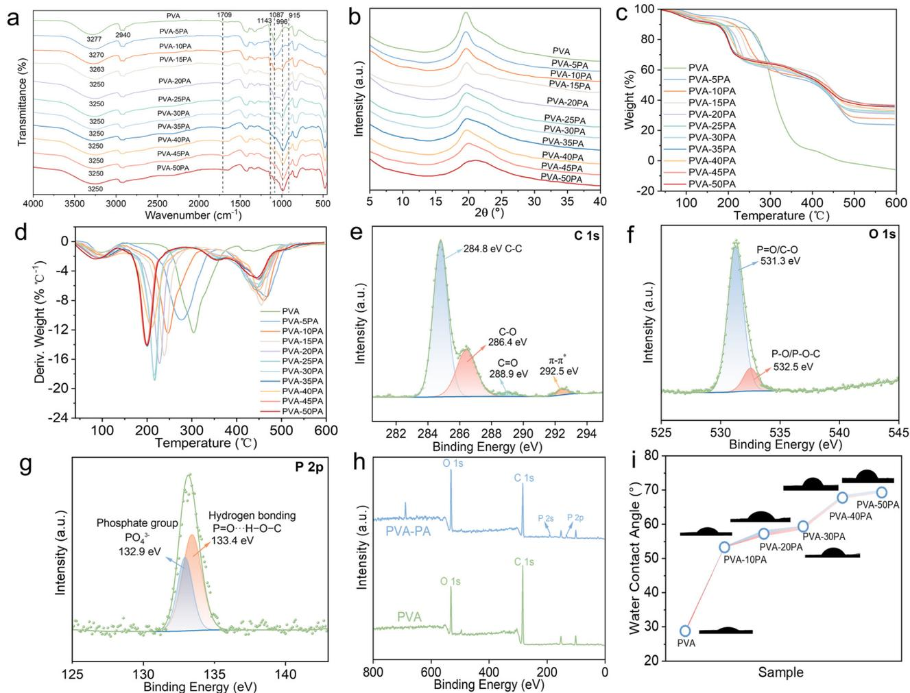
**Fig. 2** Structural and surface characterization of the PVA-PA composite films: (a–d) FTIR spectra, XRD patterns, TGA curves, and DTG curves of PVA-PA with different PA contents, respectively; (e–g) C 1s, O 1s, and P 2p XPS spectra of PVA-20PA; (h) overall XPS spectra of PVA-20PA and PVA; and (i) water contact angles (WCAs) of PVA and the PVA-PA samples with various PA percentages.
