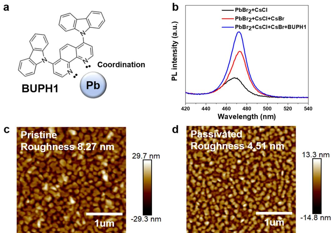
**Fig. 1** Overview of the passivation effects of BUPH1. (a) Schematic of bidentate coordination between BUPH1 and under-coordinated Pb<sup>2+</sup> ions; (b) PL spectra showing emission redshift, PLQY enhancement, and FWHM narrowing with CsBr and BUPH1; AFM images of (c) pristine and (d) BUPH1-passivated films.
