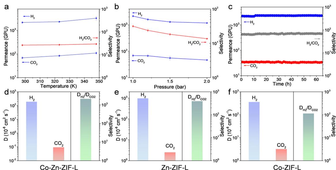
Fig. 5 The H<sub>2</sub>/CO<sub>2</sub> separation performance of the Co-Zn-ZIF-L membrane at different operation temperatures (a) and pressures (b). (c) Operational stability of the Co-Zn-ZIF-L membrane for H<sub>2</sub>/CO<sub>2</sub> separation. Feed pressure, 1.0 bar; temperature, 298 K; H<sub>2</sub>:CO<sub>2</sub>, 1:1. The diffusion coefficient of (d) Co-Zn-ZIF-L, (e) Zn-ZIF-L and (f) Co-ZIF-L for H<sub>2</sub> and CO<sub>2</sub> calculated by molecular dynamics simulation.
