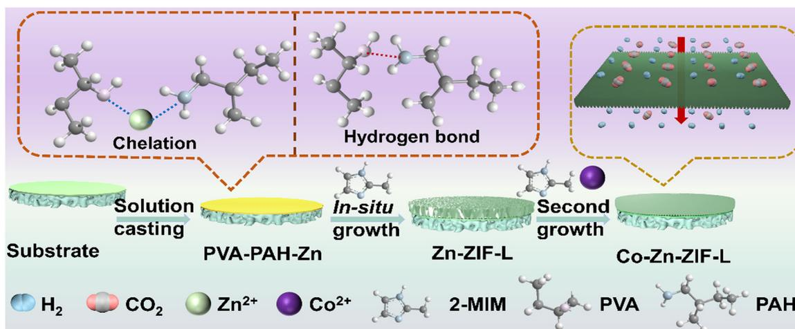
Fig. 1 Schematic of the preparation of the Co-Zn-ZIF-L membrane.
