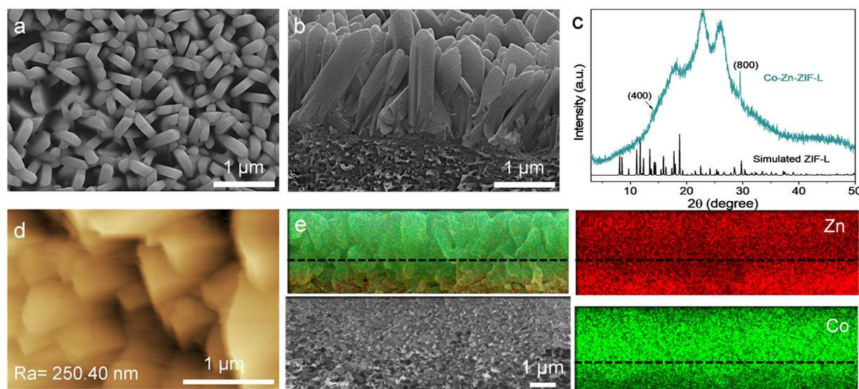
**Fig. 2** Surface (a) and cross-sectional (b) SEM images of the Co-Zn-ZIF-L membrane. (c) Simulated and experimental XRD patterns of the Co-Zn-ZIF-L membrane. (d) AFM image of the Co-Zn-ZIF-L membrane. (e) EDS image of the Co-Zn-ZIF-L membrane.
