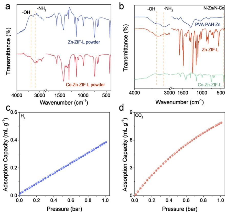
Fig. 3 (a) ATR-FTIR spectrum of Zn-ZIF-L and Co-Zn-ZIF-L powders; (b) ATR-FTIR spectrum of PVA-PAH-Zn, Zn-ZIF-L and Co-Zn-ZIF-L membranes; the adsorption isotherms of Co-Zn-ZIF-L powder for H<sub>2</sub> (c) and CO<sub>2</sub> (d) at 303 K.
