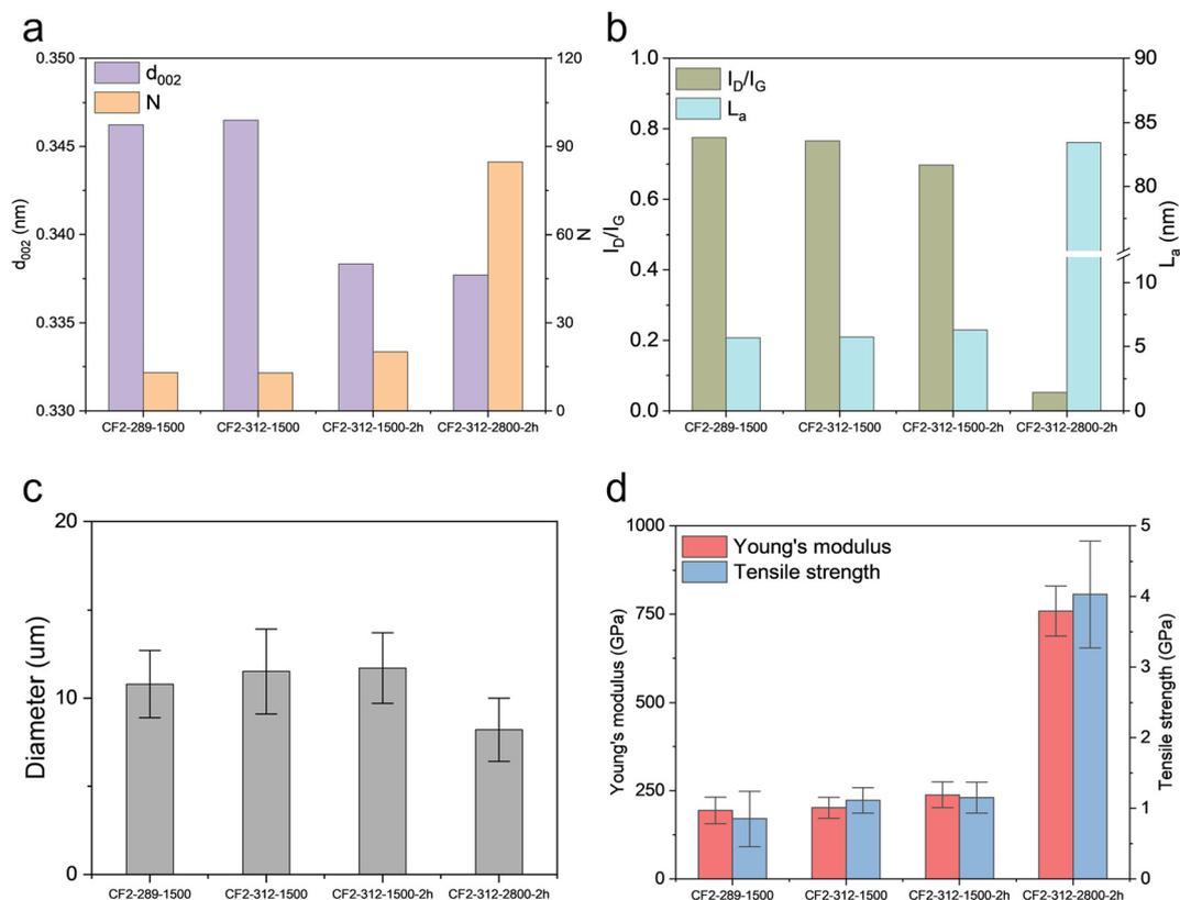
**Fig. 9** Crystalline data, diameters, and mechanical properties of different heat-treatment conditions. (a)  $d_{002}$  and quantity of stacked layers ( $N$ ) extracted from XRD pattern; (b) ratio of  $l_D$  to  $l_G$  ( $l_D/l_G$ ) and in-plane crystalline size ( $L_a$ ) extracted from Raman spectra; (c) diameters of CFs; (d) Young's modulus and tensile strength.
