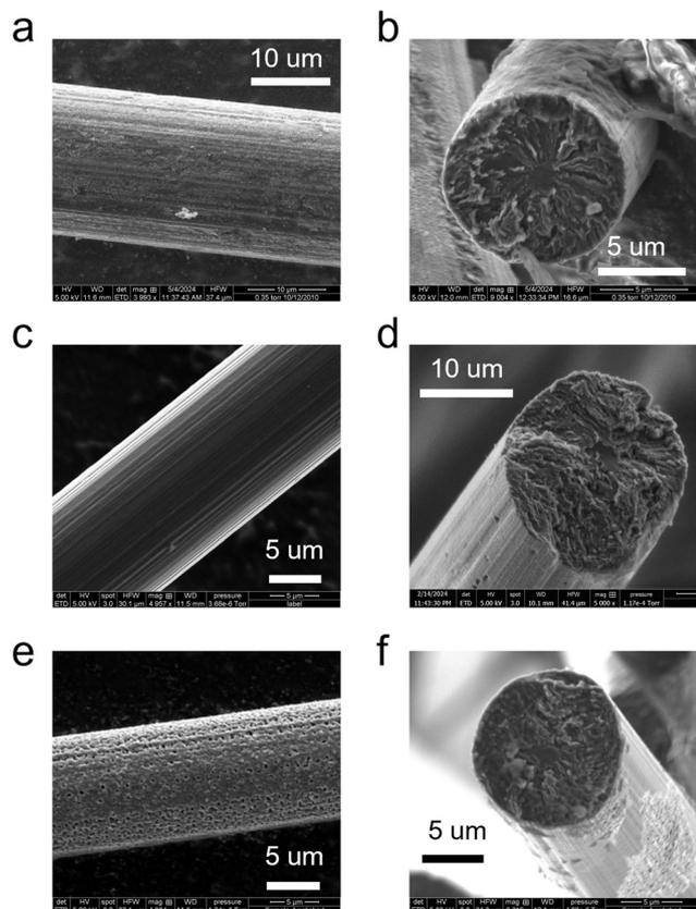
Fig. 7 SEM images of CFs. Column 1: side view, column 2: cross-section view. (a) and (b): CF2-266-1500; (c) and (d): CF2-312-1500; (e) and (f): CF2-335-1500. CF2-289-1500 is shown in Fig. 5c and d.
