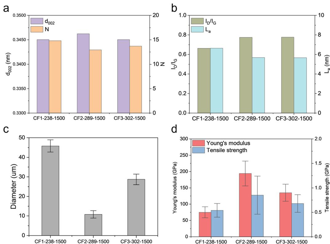
**Fig. 6** Crystalline data, diameters, and mechanical properties of CFs fabricated from different MCPLs. (a)  $d_{002}$  and quantity of stacked layers (N) extracted from XRD pattern; (b) ratio of  $I_D$  to  $I_G$  ( $I_D/I_G$ ) and in-plane crystalline size ( $L_a$ ) extracted from Raman spectra; (c) diameters of CFs; (d) Young's modulus and tensile strength.
