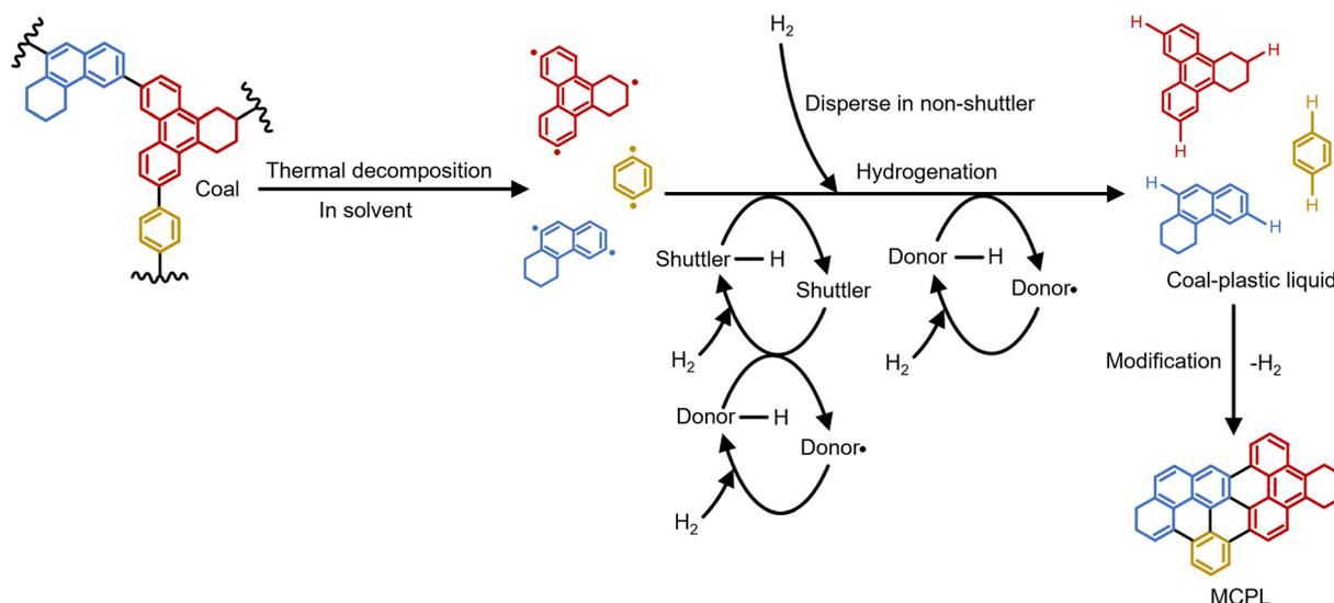
**Fig. 10** Proposed mechanisms of mild solvolysis liquefaction.
