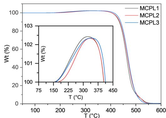
Fig. 2 TGA curves of MCPL1–3. Inset: Detail from 100–450 °C (method: under airflow, ramped at 0.5 °C min<sup>-1</sup> from room temperature to 600 °C, and held at 600 °C for 2 h).
