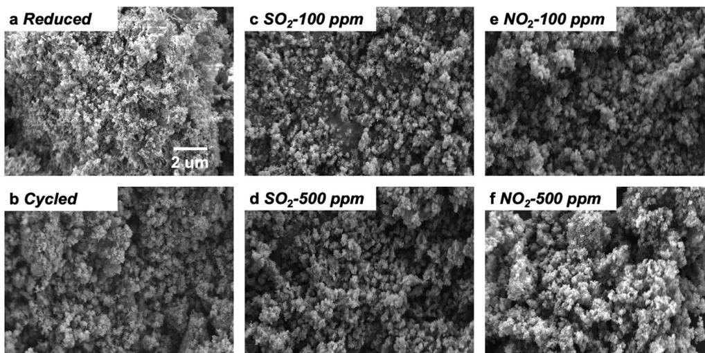
Fig. 9 SEM images of pre-reduced and cycled Ni5Al15Ca DFMs. (a) Pre-reduced DFM, (b) cycled DFM without SO<sub>2</sub> or NO<sub>2</sub>, (c) cycled DFM with 100 ppm SO<sub>2</sub>-containing flue gas, (d) cycled DFM with 500 ppm SO<sub>2</sub>-containing flue gas, (e) cycled DFM with 100 ppm NO<sub>2</sub>-containing flue gas, and (f) cycled DFM with 500 ppm NO<sub>2</sub>-containing flue gas.
