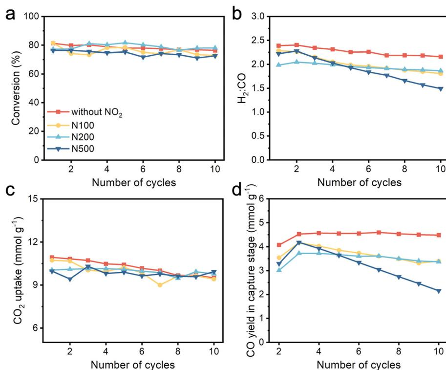
Fig. 4 Cyclic performance of ICCU-DRM under  $NO_2$ -containing flue gas conditions. (a)  $CO_2$  conversion, (b)  $H_2:CO$  ratio, (c)  $CO_2$  uptake and (d)  $CO$  yield in the capture stage. N100 refers to the cycled DFM with 100 ppm  $NO_2$  in flue gas.
