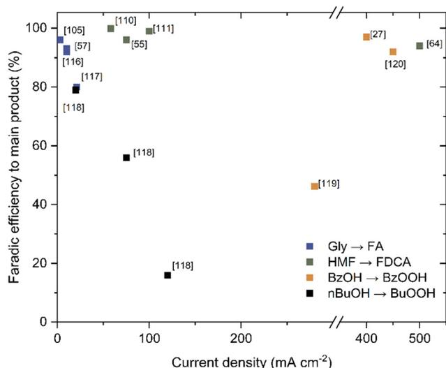
**Fig. 4** Faradaic efficiencies and associated current densities for various alcohol oxidation catalyzed by electrocatalysts based on earth-abundant materials.<sup>27,55,57,64,105,110,111,116–120</sup> Abbreviations: Gly: glycerol; FA: formic acid; HMF: hydroxymethylfurfural; FDCA: 2,5-furandicarboxylic acid; BzOH: benzyl alcohol; BzOOH: benzoic acid; *n*-BuOH: 1-butanol; BuOOH: butanoic acid.
