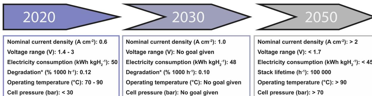
Fig. 2 A timeline of the technical advancements related to alkaline water electrolysis proposed by the International Renewable Energy Agency (IRENA),<sup>2</sup> the Joint Hydrogen Undertaking (JHU) developed by European Clean Hydrogen Partnership (ECHP),<sup>10</sup> and an overview of the state of the art as given by the JHU and IRENA in 2020. \*Degradation is defined here as the energy efficiency loss when running at nominal capacity for a given time.
