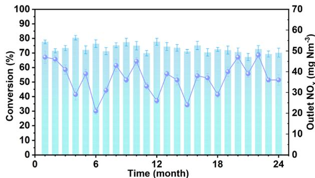
Fig. 11 Industrial application of the plate-type 3%V<sub>2</sub>O<sub>5</sub>-10%MoO<sub>3</sub>/TiO<sub>2</sub> catalyst. Bars: monthly average conversion; line with symbols: concentration of outlet NO<sub>x</sub>. For detailed work conditions, see the Experimental section.
