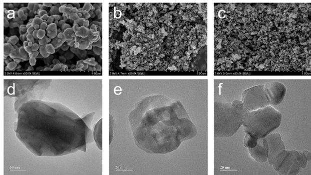
**Fig. 3** SEM images of (a) rutile TiO<sub>2</sub>, (b) anatase TiO<sub>2</sub> and (c) P25 TiO<sub>2</sub> supported catalysts; and TEM images of (d) rutile TiO<sub>2</sub>, (e) anatase TiO<sub>2</sub> and (f) P25 TiO<sub>2</sub> supported catalysts.
