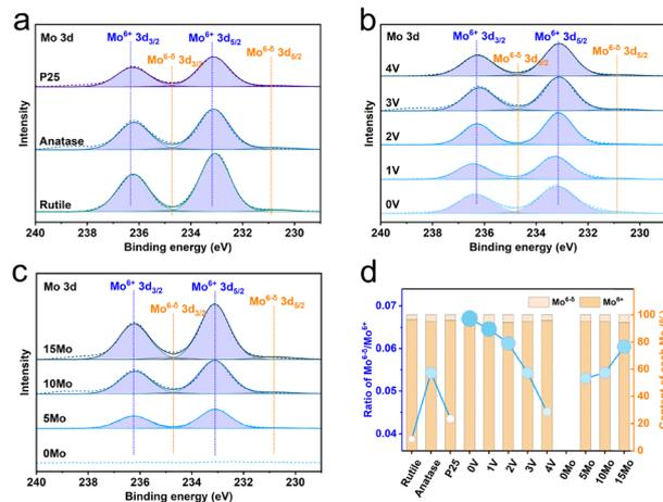
Fig. 5 (a–c) XPS spectra of Mo 3d and (d) ratio of Mo<sup>6-δ</sup>/Mo<sup>6+</sup> and content of each Mo in different catalysts.
