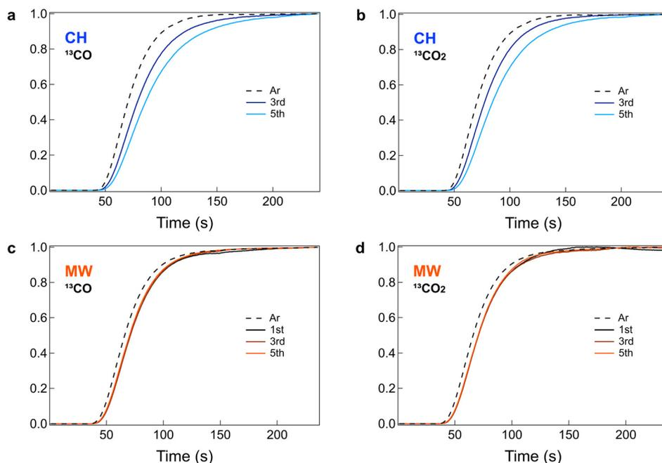
**Fig. 2** Normalised and overlaid 3rd and 5th switches for the MS signals of (a) CO and (b) CO<sub>2</sub> under conventional heating at 600 °C and 1st, 3rd, and 5th switches for the MS signals of (c) CO and (d) CO<sub>2</sub> under microwave heating at 490 °C under the condition of CH<sub>4</sub>:CO<sub>2</sub> = 2:1. Owing to the dynamically changing response during the 1st switch, the reactant (CO<sub>2</sub>) and product (CO) responses of the switch are not shown in (a) and (b).
