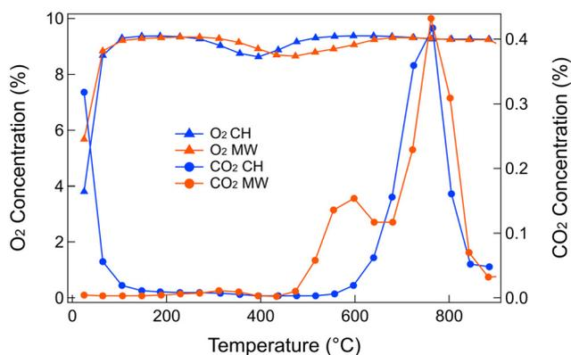
Fig. 5 O<sub>2</sub> and CO<sub>2</sub> concentrations during TPO over the spent catalyst after conventional heating (CH) and microwave heating (MW) at CH<sub>4</sub>:CO<sub>2</sub> = 1:1. Gas composition = 10% O<sub>2</sub>-He balance, flow rate = 50 mL min<sup>-1</sup>, temperature range = R. T. to 900 °C, and heating rate = 10 °C min<sup>-1</sup>.
