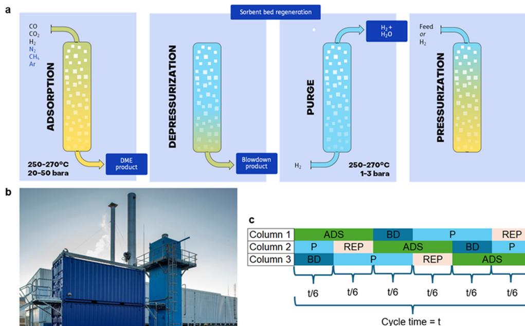
**Fig. 10** Steps of the SEDMES process operating as a pressure swing regeneration unit – PSA (a); SEDMES pilot plant at TNO, Petten, The Netherlands, designed to produce 3 kg<sub>DME</sub> h<sup>-1</sup> (b) and cycle design operating in the pilot plant (c).
