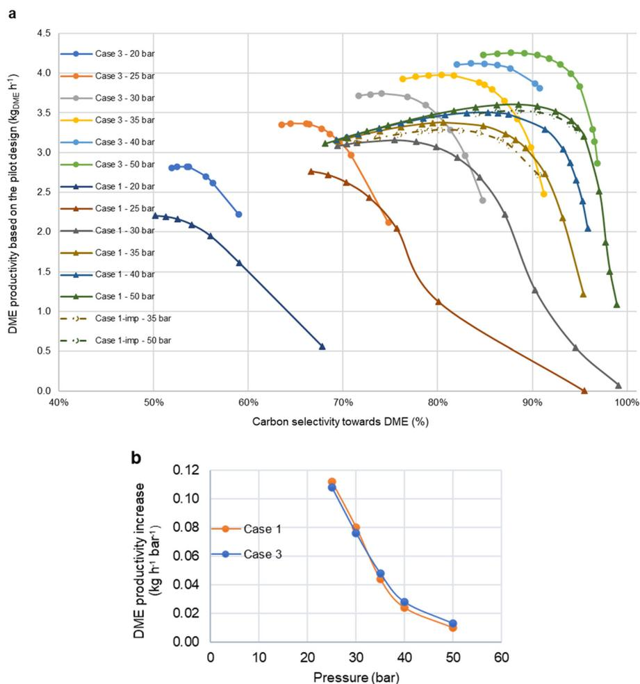
**Fig. 1** Comparison of DME productivity and selectivity for cases 1 and 3, for different operating pressures and cycle durations (cycle duration increases while moving to lower carbon selectivity) (a); rate of DME productivity increase per unit of pressure (b); the reaction temperature is 250 °C.
