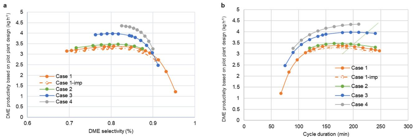
**Fig. 3** Pareto plot of DME productivity vs. DME selectivity with lower DME selectivity (left side of the x-axis) corresponding to increasing cycle duration (a); DME productivity against cycle duration showing the maximum operating points with the green line (b). Dashed lines show the performance of case 1 in case it contained a similar level of impurities to the other cases.
