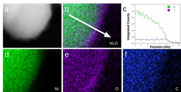
Fig. 4 Post *in situ* STEM-EDS analysis of the catalyst nanoparticle showing the annular dark-field STEM (a), Ni, O EDS overlay map (b), variation of Ni and O count along the arrow direction (c), and corresponding Ni (d), O (e), and C (f) EDS map.
