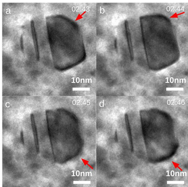
**Fig. 2** *In situ* time-series of TEM images showing a dynamic active particle away from the edge of the carbon support, from time 2:43 to 2:46 (a–d). The area that has undergone dynamic changes is indicated by the red arrows.
