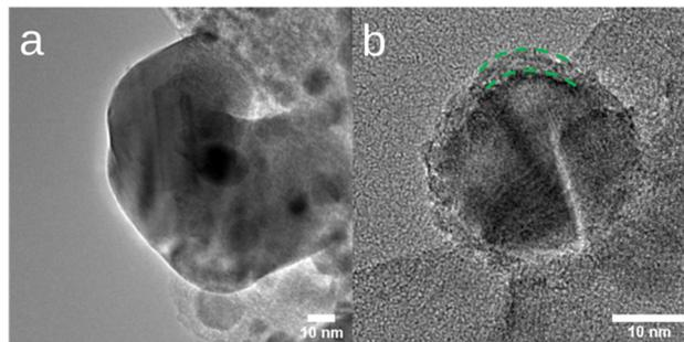
Fig. 1 The *ex situ* TEM analysis results of the Ni/ACR catalyst before (a) and after (b) CO<sub>2</sub> methanation for 90 h. The resultant Ni@NiO core@shell nanostructure is highlighted by the green dashed lines in (b).
