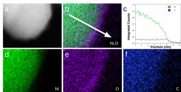
Fig. 4 Post *in situ* STEM-EDS analysis of the catalyst nanoparticle showing the annular dark-field STEM (a), Ni, O EDS overlay map (b), variation of Ni and O count along the arrow direction (c), and corresponding Ni (d), O (e), and C (f) EDS map.
