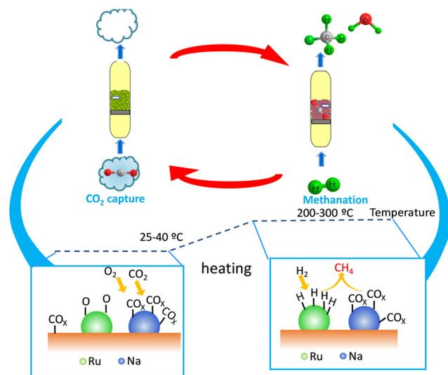
**Fig. 2** A scheme of the mechanism of CO<sub>2</sub> capture from air and methanation. Top: macroscopic scale; bottom: mechanism at the nanoscopic scale of DFM.
