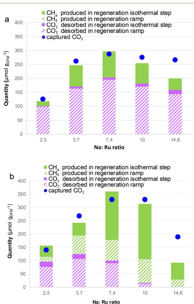
**Fig. 6** The effect of different Na:Ru ratios on the captured CO<sub>2</sub> and produced CH<sub>4</sub> and CO<sub>2</sub> in regeneration. Capture from humid air at 40 °C and regeneration at 200 °C following method A (a) and method B (b). DFM mass = 70 mg, total flow rate = 60 mL min<sup>-1</sup>, and cycle number = 4.
