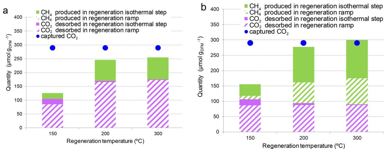
**Fig. 4** Effect of the temperature of the second step (regeneration) on gas composition and CO<sub>2</sub> capture: (a) method A, heating in Ar flow and feeding H<sub>2</sub> at the set-point temperature for 30 min; (b) method B, heating in 20% H<sub>2</sub> in Ar at the set-point temperature and holding for 30 min. The capture is performed under dry air at 40 °C using the DFM NaRu (3.7 : 1). DFM mass = 70 mg, flow rate = 60 mL min<sup>-1</sup>, and cycle number = 4.
