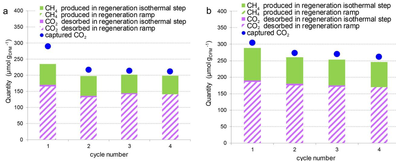
**Fig. 5** Four cycles of CO<sub>2</sub> capture at 40 °C under dry air (a) and under humid air (b), and regeneration at 200 °C following method A for DFM NaRu (3.7 : 1). DFM mass = 70 mg, and total flow rate = 60 mL min<sup>-1</sup>.
