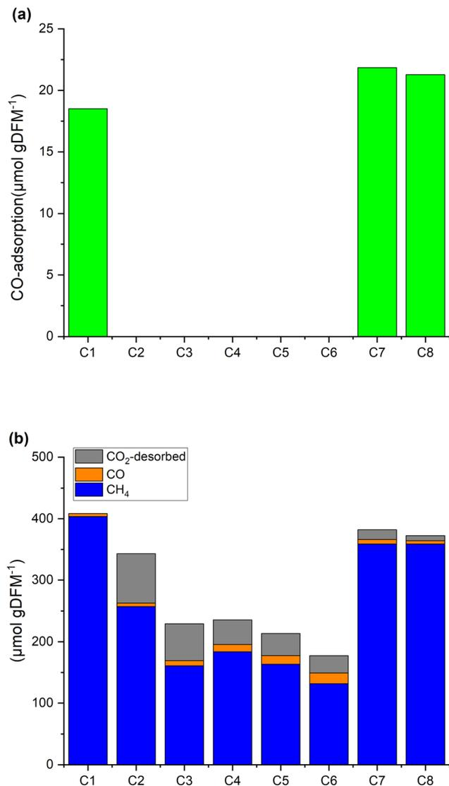
**Fig. 13** Produced gases during hydrogenation in ideal and realistic cyclic testing with 15Ni1Ru, 7.9Na/Al, ideal adsorption step: 10% CO<sub>2</sub>/N<sub>2</sub>, realistic adsorption step: 10%CO<sub>2</sub> + 2.7%O<sub>2</sub> + 2.9%H<sub>2</sub>O/Ar, hydrogenation step: 10% H<sub>2</sub>/N<sub>2</sub>, at 400 °C.
