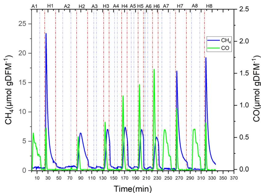
Fig. 12 Dynamic curves of ideal and realistic cyclic testing with 15Ni1Ru, 7.9Na/Al, ideal adsorption step: 10% CO<sub>2</sub>/N<sub>2</sub>, realistic adsorption step: 10%CO<sub>2</sub> + 2.7%O<sub>2</sub> + 2.9%H<sub>2</sub>O/Ar, hydrogenation step: 10% H<sub>2</sub>/N<sub>2</sub>, at 400 °C.
