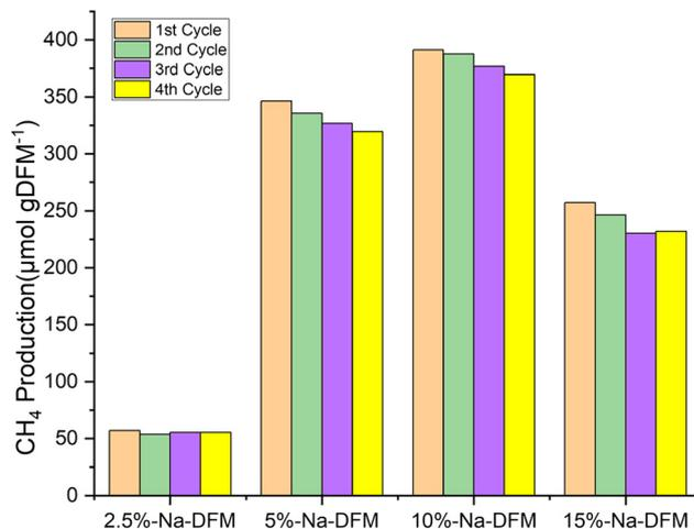
Fig. 8 CH<sub>4</sub> production during the hydrogenation step for 15Ni1Ru, XNa-DFMs (X = 2.5–15%), at 400 °C, with 10H<sub>2</sub>/N<sub>2</sub> (50 mL min<sup>-1</sup>) in hydrogenation step – 15 minutes.
