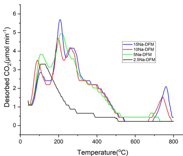
**Fig. 5**  $\text{CO}_2$ -TPD profiles of 15Ni1Ru, XNa-DFMs ( $X = 2.5\text{--}15\%$ ), with 10%  $\text{CO}_2/\text{N}_2$  ( $50 \text{ mL min}^{-1}$ ), 40–800 °C.**Table 3** Weak, medium, and strong basic sites 15Ni1RuXNa-DFMs ( $X = 2.5\text{--}15\%$ )
