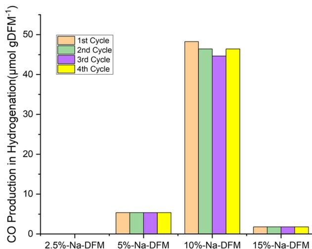
Fig. 9 CO production during the hydrogenation step 15Ni1Ru, XNa-DFMs (X = 2.5–15%), at 400 °C, with 10H<sub>2</sub>/N<sub>2</sub> (50 mL min<sup>-1</sup>) in hydrogenation step – 15 minutes.
