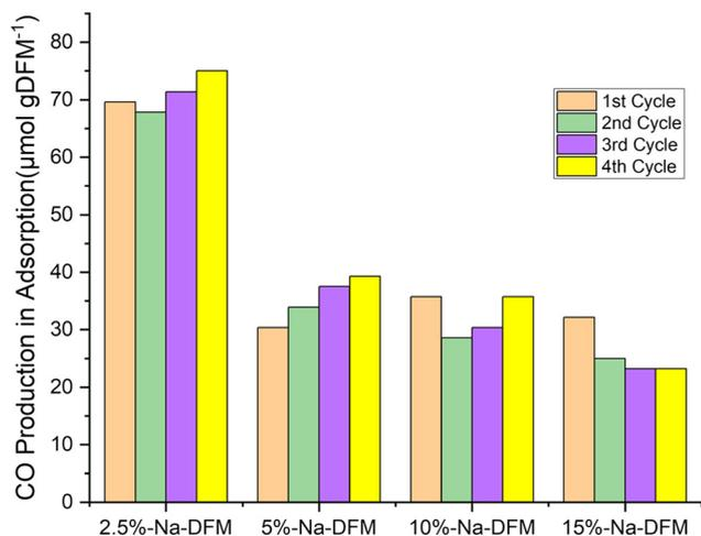
Fig. 7 CO production during the adsorption step for 15Ni1Ru, XNa-DFMs (X = 2.5–15%), at 400 °C, with 10% CO<sub>2</sub>/N<sub>2</sub> (50 mL min<sup>-1</sup>) in adsorption step – 15 minutes.
