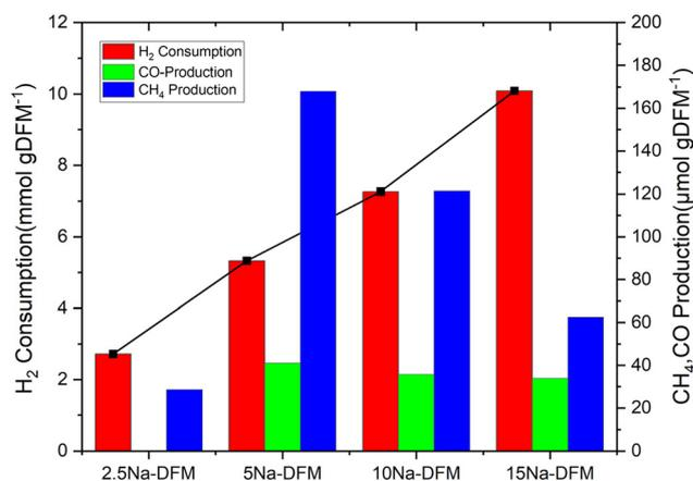
**Fig. 6** Total  $\text{H}_2$  consumption,  $\text{CH}_4$  production and  $\text{CO}$  production of 15Ni1Ru, XNa-DFMs ( $X = 2.5\text{--}15\%$ ) during  $\text{H}_2$ -TPSR, with 10%  $\text{H}_2/\text{N}_2$  ( $50 \text{ mL min}^{-1}$ ), 25–900 °C.
