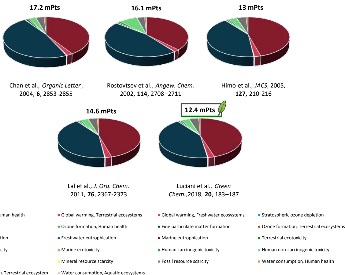
Fig. 10 Endpoint comparison through the investigated methodologies (ReCiPe 2016, influence of the impact categories on the single score).
