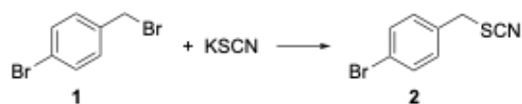
Scheme 1 Reaction of 4-bromobenzylbromide ( 1 , 50.0 mg, 0.2 mmol) with potassium thiocyanate (58.3 mg, 0.3 mmol, 3 equiv.) to give 4-bromobenzylthiocyanate ( 2 ).
