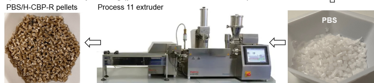
Fig. 1 Schematic representation of the valorization process for Consolidated Bioprocessing residuals (CBP-R) into bio-composite pellets. (A) Mechanical size reduction of CBP-R is carried out using a cyclone mill (CM) followed by high-shear homogenization (HSH) then spray dried. (B) Dry homogenized CBP residuals (H-CBP-R) are compounded with poly(butylene succinate) (PBS) pellets in a melt twin-screw extruder to yield bio-composite pellets.
