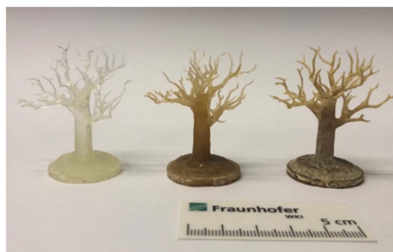
Fig. 9 Printed parts from wood and olive kernel flour-based materials, neat material, materials with olive kernel flour and wood flour (left to right). 108 Reproduced from the open-access journal Reactive and Functional Polymers .
