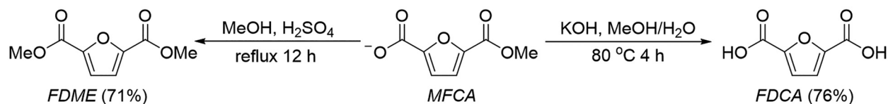
Scheme 2 Synthesis of FDME and FDCA from MFCA via esterification and hydrolysis, respectively.
