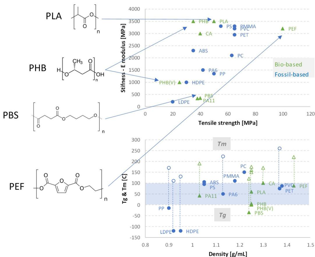
Fig. 7 Sugar-based polymers (green) can provide a variety of properties already offered by today's fossil polymers (blue) ( $T_g$  and  $T_m$  represent the glass transition and melting temperatures of polymers; adapted from ref. 25).
