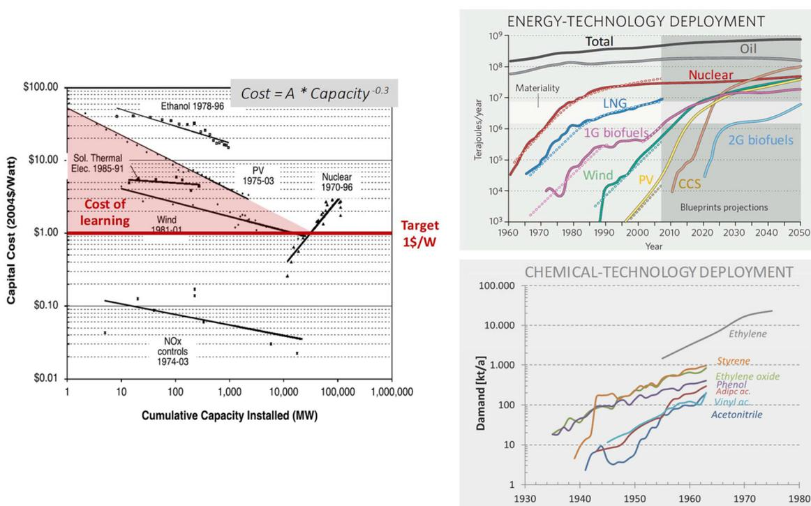
**Fig. 14** Technology maturation erodes the manufacturing costs (left) but takes about half a century to complete (top and bottom right) (top left and right adapted from ref. 62 and 65 with permission from Springer, copyright 2007 and 2009; bottom right with data sourced from ref. 63 and 64).
