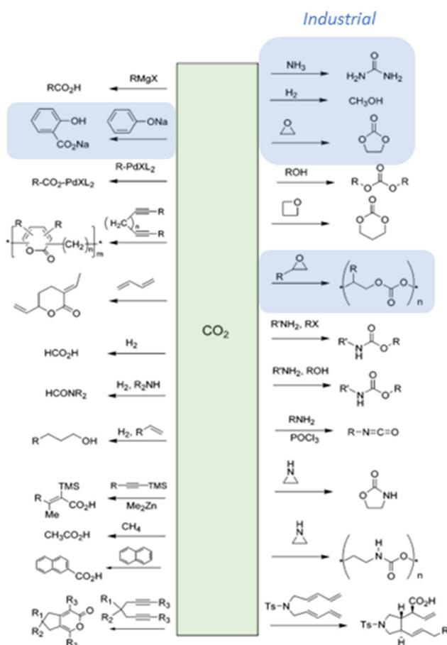
**Fig. 9** Approaches to CO<sub>2</sub> valorisation (adapted from ref. 45 with permission from *Chem. Rev.*, copyright 2007).
