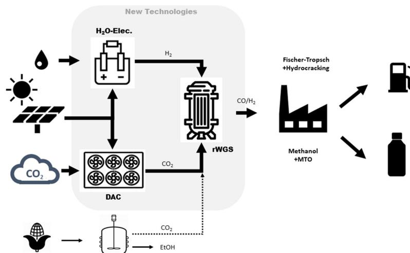
Fig. 10 Portfolio of technologies for CO<sub>2</sub> capture and hydrogenation.
