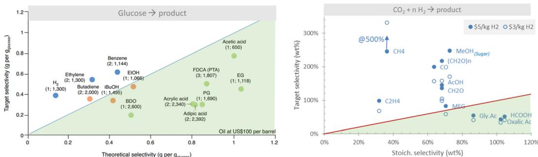
**Fig. 12** Screening economics for valorising sugars and  $\text{CO}_2$  (premise: glucose at \$300 per t,  $\text{CO}_2$  at \$100 per t,  $\text{H}_2$  at \$3–5 per kg; \$200 per t per step; multiple steps for glucose but single step for  $\text{CO}_2$ ; bottom left comes from ref. 17).
