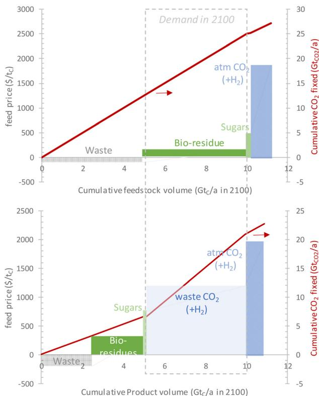
**Fig. 4** Potential volume, costs and GHG emissions of renewable carbon feedstocks (top) and their derived products (bottom) after correction for conversion yields. The carbon lost during the conversion of waste, sugar and biomass forms the waste CO<sub>2</sub> feedstock (premises are detailed in the text).
