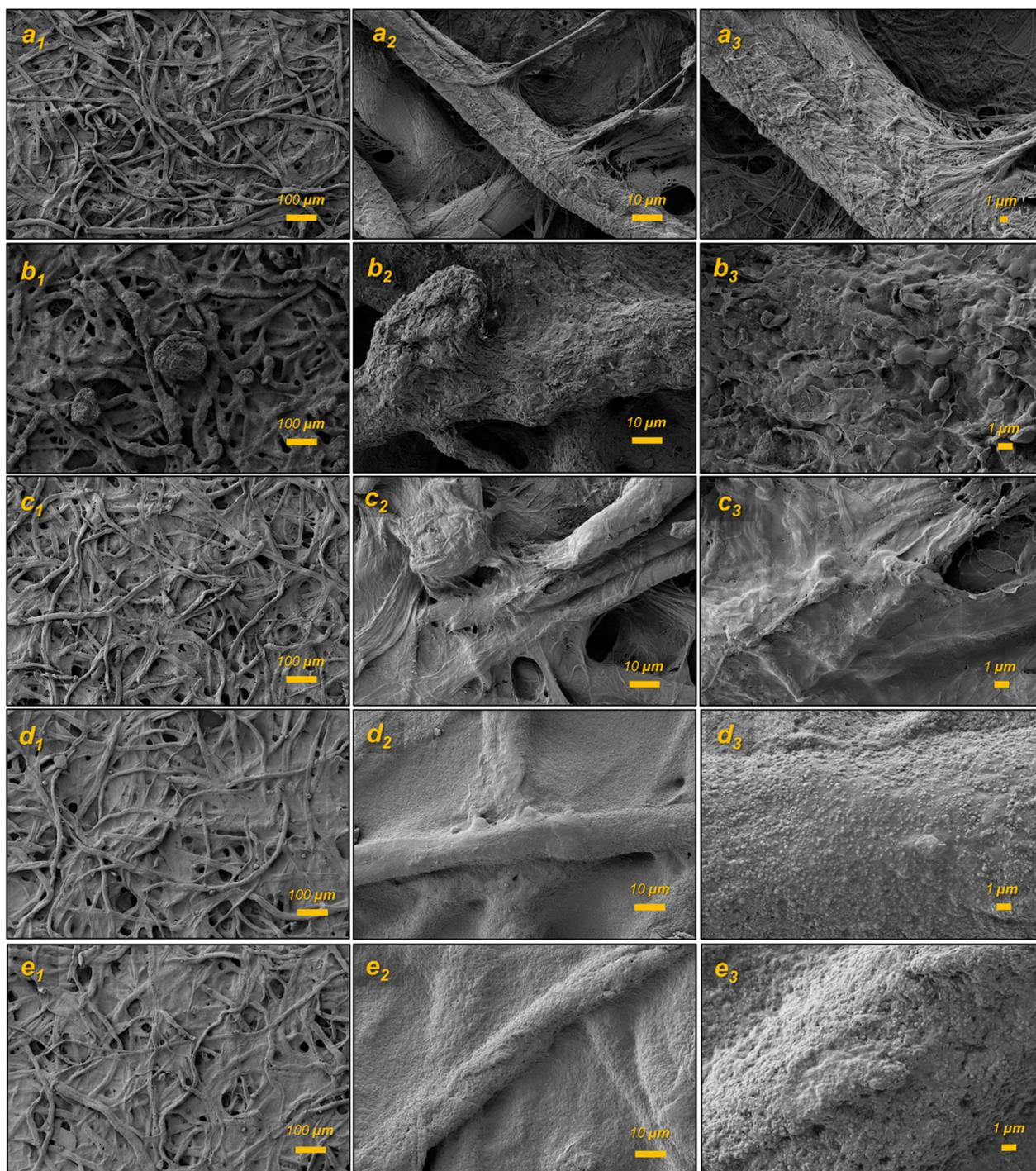
Fig. 4 SEM images of the surface of filter paper: (a) uncoated, (b and c) acetone-based p-lignin (b: no curing, c: oven-cured), and (d and e) waterborne p-lignin (d: 0.4% HEC, e: 1% HEC).
