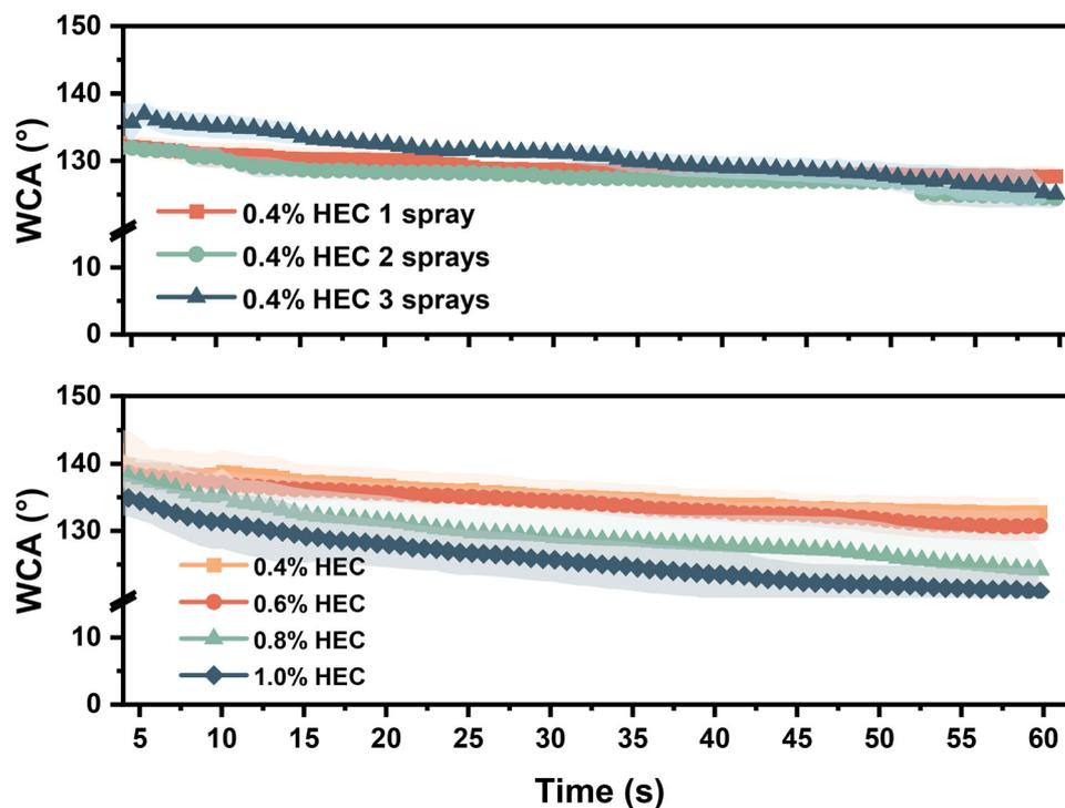
Fig. 6 Water contact angle (WCA) of waterborne p-lignin spray over 60 s: effect of spray cycles at 0.4% HEC (top) and effect of HEC loading at three spray cycles (bottom).
