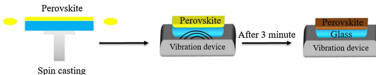
Fig. 12 Ultrasonic vibration annealing, reproduced from ref. 175 with permission from Elsevier. 175 Copyright 2018.
