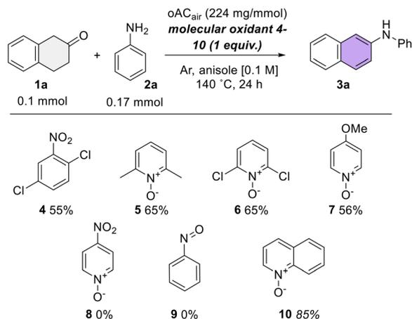
**Fig. 2** Screening of various molecular oxidants, reaction conditions: catalyst loading (defined as 1 equiv.) 224 mg mmol<sup>-1</sup>, 0.1 mmol **1a**, 0.17 mmol **2a**, 0.1 mmol molecular oxidant in 1 mL of anisole.
