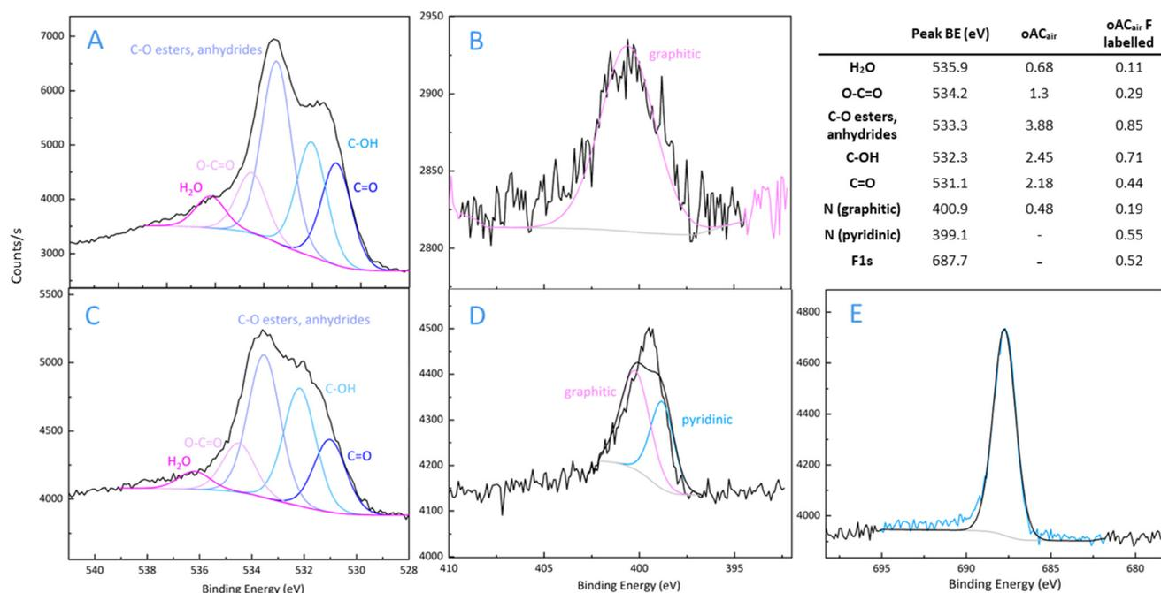
**Fig. 4** XPS analysis of oAC<sub>air</sub> before and after 4,5-difluorobenzene-1,2-diamine labelling: summary of O1s deconvolutions (a) and (c), N 1s (b) and (d) and F 1s (e) peaks. Atomic values in Table in %.
