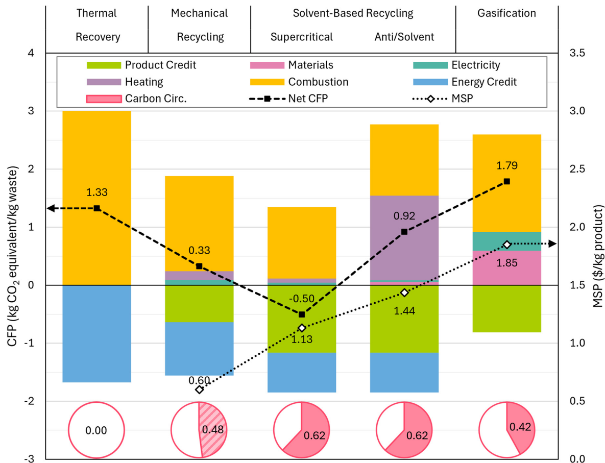
Fig. 4 Comparison of gasification to other polyolefin disposal routes, including thermal recovery, mechanical recycling, and solvent-based recycling. CFP and contributing emissions are on the left axis, MSP on the right axis, and Carbon Circularity is represented with pie charts beneath each column.
