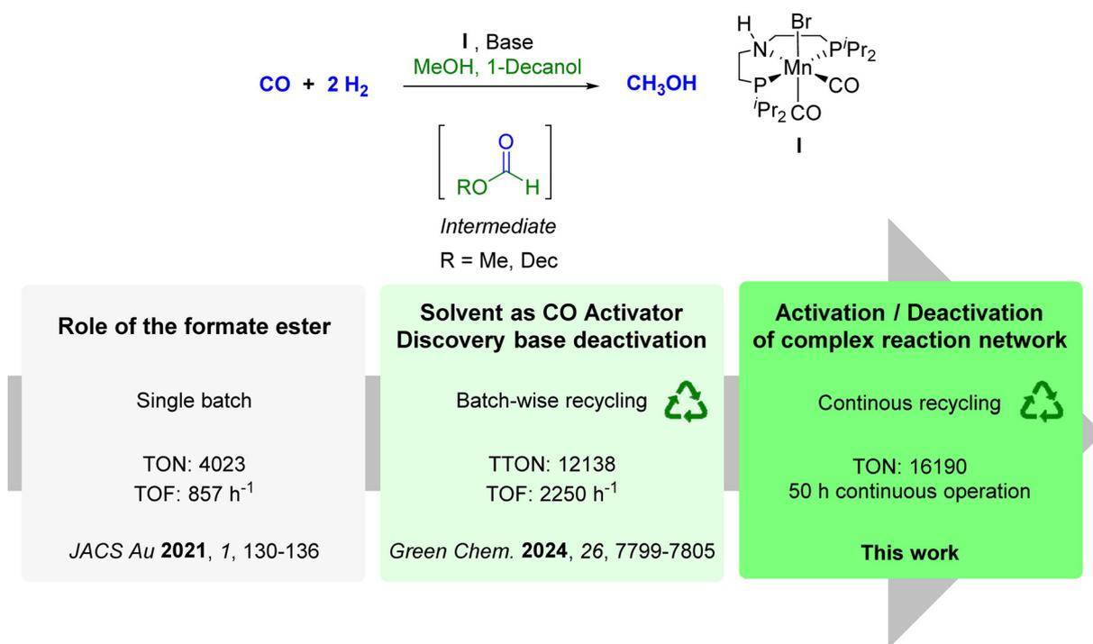
**Fig. 1** Development of alcohol-assisted carbon monoxide hydrogenation to methanol with manganese pincer catalyst **I** from mechanistic understanding to continuous operation.<sup>35,40</sup>
