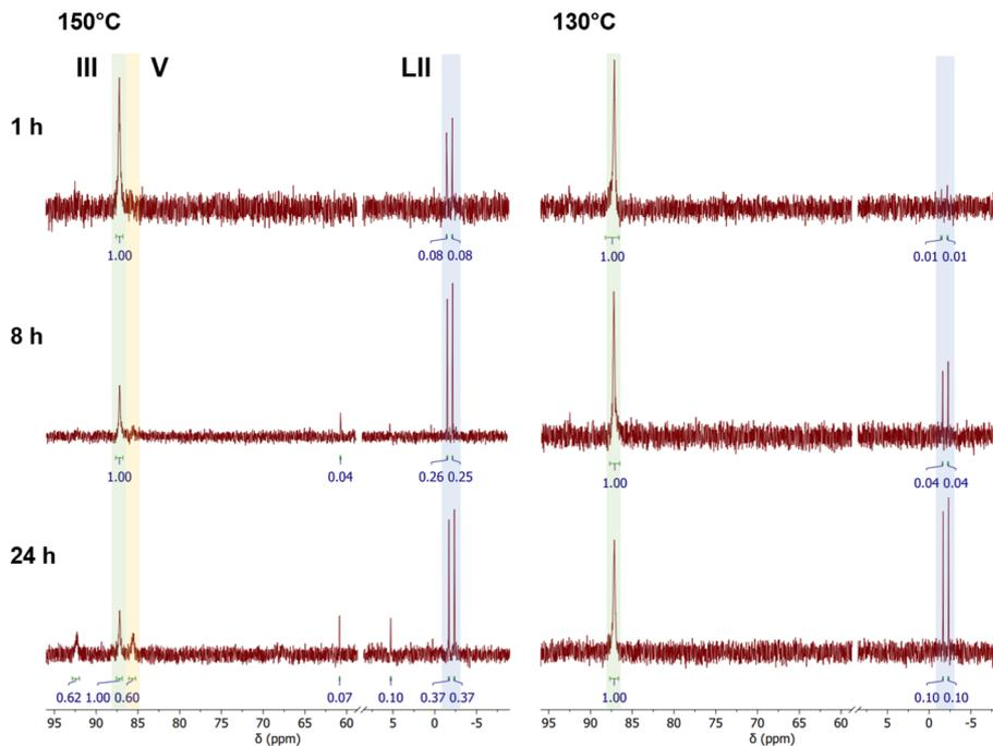
Fig. 4  $^{31}\text{P}$ -NMR (162 MHz, methanol) spectra of the reaction at 150 °C and 30 bar (left) and the reaction at 130 °C, 60 bar (right) after 1 h, 8 h and 24 h.  $\delta = -1.8$  (blue, free Ligand LII), 85.6 (yellow, dormant species V), 87.1 (green, active catalyst III), and 92.3 (deactivated species) ppm.
