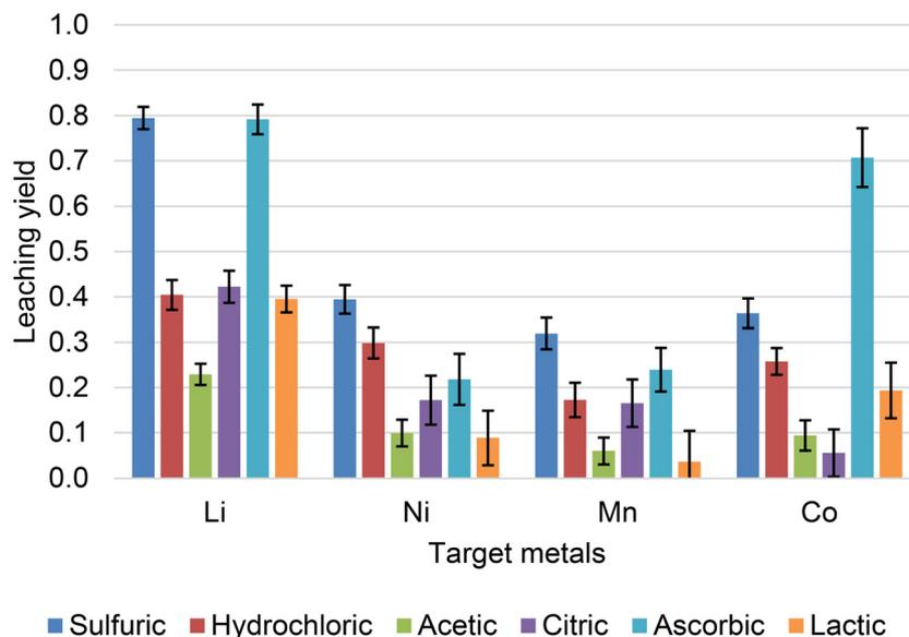
**Fig. 10** Metal leaching yields from NMC111 predicted by the developed PD-GBR model for fixed conditions: 40 °C, 50 g L<sup>-1</sup>, 60 min leaching, 1 mol L<sup>-1</sup> of acid.
