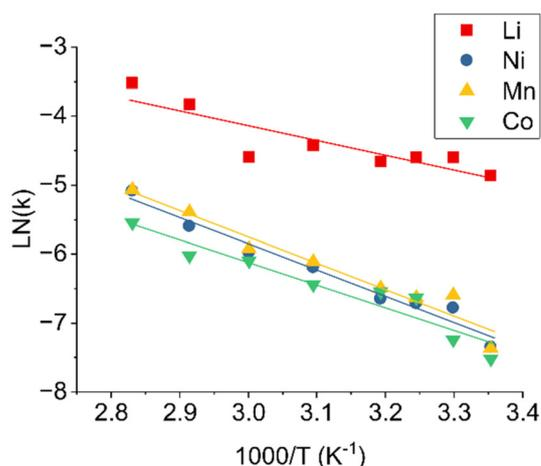
**Fig. 9** Arrhenius plot for the leaching of Li, Ni, Mn, and Co from NMC111 cathodes between 25–80 °C. The slopes of the linear regression are used to calculate the activation energies ( $E_a$ ) presented in Table 3. The simulated kinetics data used to compute the kinetic parameters are available in Fig. S3 of the SI.
