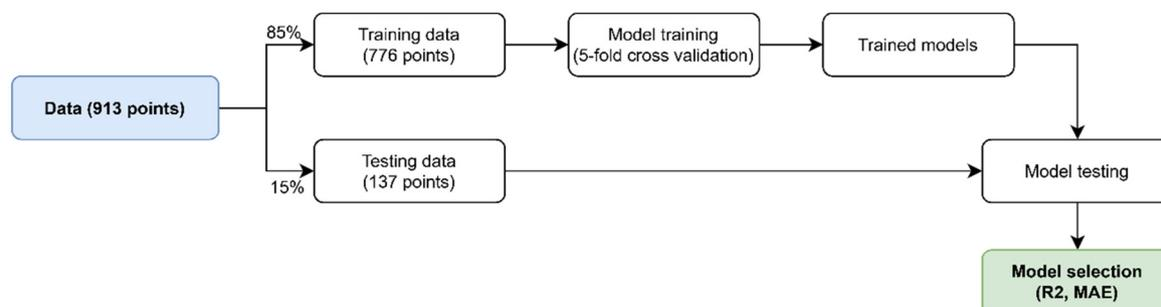
Fig. 1 Simplified data flow chart for model training and selection.
