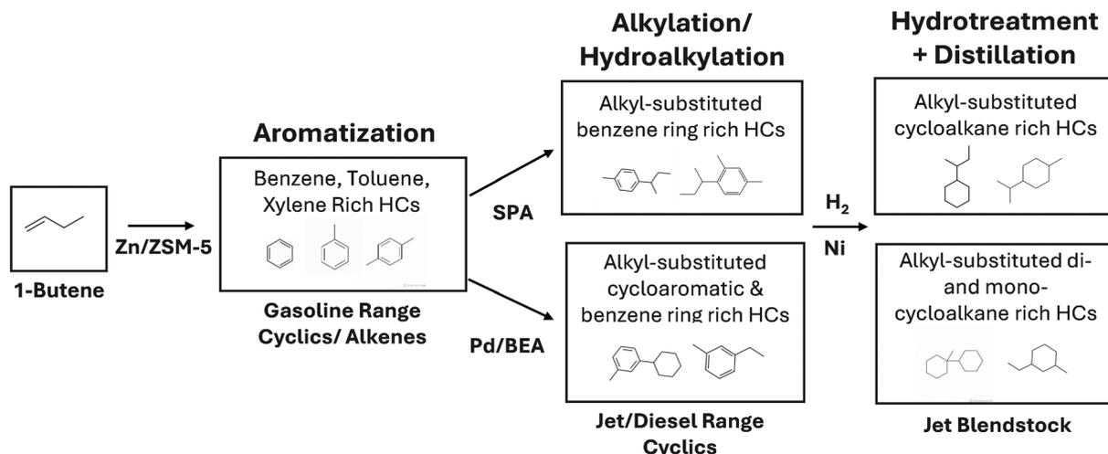
**Fig. 7** Simplified process flow diagram for the two approaches reported here for converting gasoline-range aromatics into either (i) alkyl-substituted cycloalkane rich hydrocarbons (HCs) or (ii) alkyl-substituted di- and mono-cycloalkane rich HCs in the jet-range.
