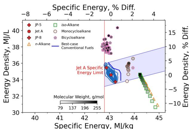
**Fig. 1** Energy density and specific energy of various fuels and hydrocarbons. The red symbols depict conventional jet fuel densities taken from the Petroleum Quality Information System database. The dark blue line represents the highest value obtained from this database. Neat hydrocarbons are also plotted for reference (ref. 3).
