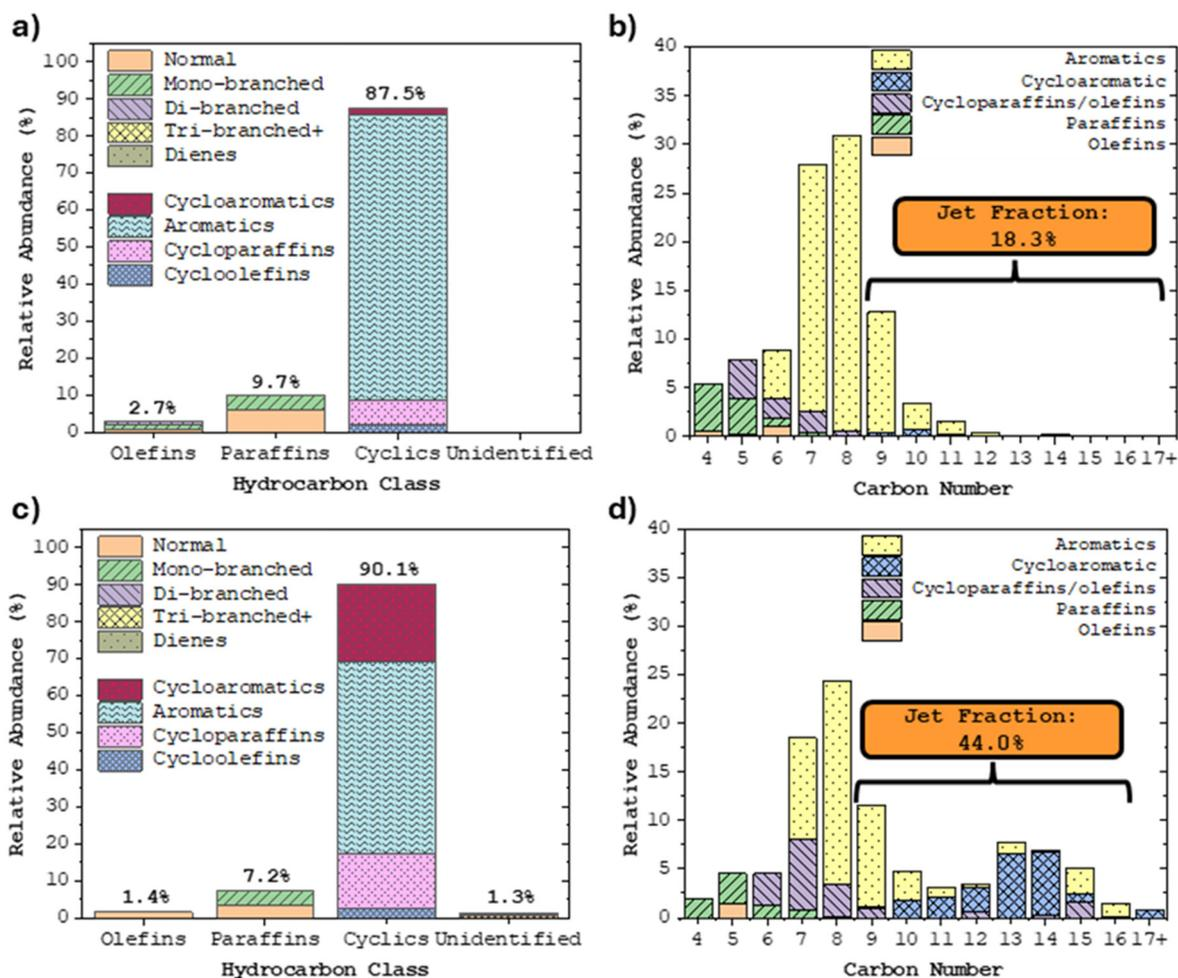
**Fig. 6** (a) Liquid product classification and (b) carbon number for the high aromatic content feed (step i, Fig. 2); (c) liquid product composition and (d) carbon number distribution for the hydroalkylation product after 6 hours' time-on-stream (step i; feed: aromatic feed/ $H_2$  = 1/1 mol; 0.15% Pd/BEA catalyst; 140 °C, 270 psig, 2.0  $h^{-1}$  WHSV).
