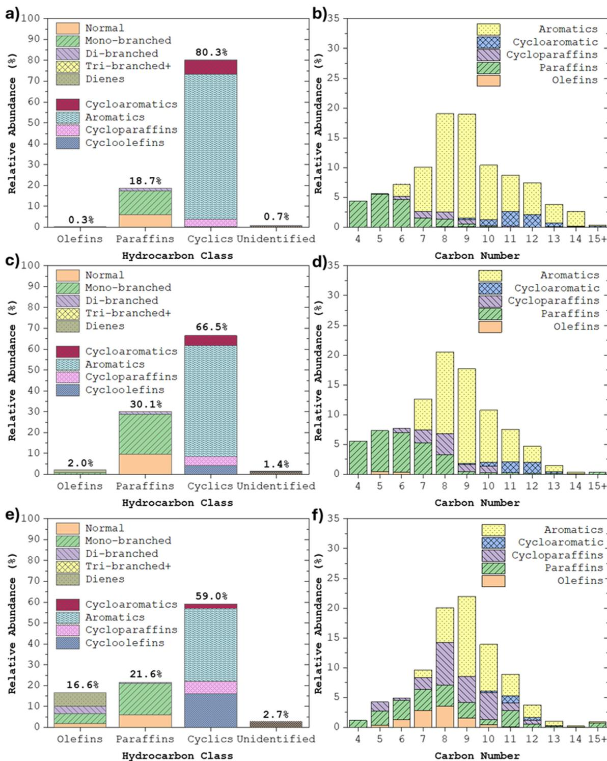
Fig. 3 Conversion of 1-butene over hydrothermally-treated 1.5%Zn/ZSM-5 ( $\text{SiO}_2/\text{Al}_2\text{O}_3 = 23$ ) and resulting (a, c and e) liquid product classification and (b, d and f) carbon number distribution at (a and b) 19, (c and d) 51, and (e and f) 76 hours' time on stream ( $T = 340^\circ\text{C}$ ,  $P = 350$  psig,  $\text{WHSV}_{1\text{-butene}} = 0.19\text{ h}^{-1}$ ; feed = 50 mol% 1-butene in  $\text{N}_2$ ).
