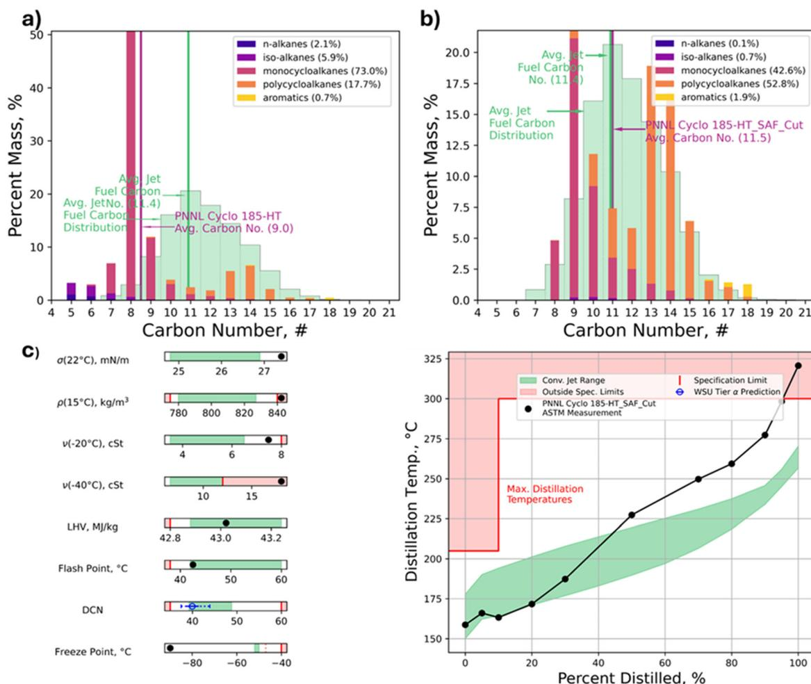
**Fig. 9** (a) Full distillate sample of the alkylated product after hydrotreatment (see Fig. S7d). (b) Jet range (>130 °C b.p. cut) after distillation. The green shaded region represents the carbon distribution of an average conventional jet fuel for reference. (c) Tier beta property measurement for the jet range hydrocarbons.
