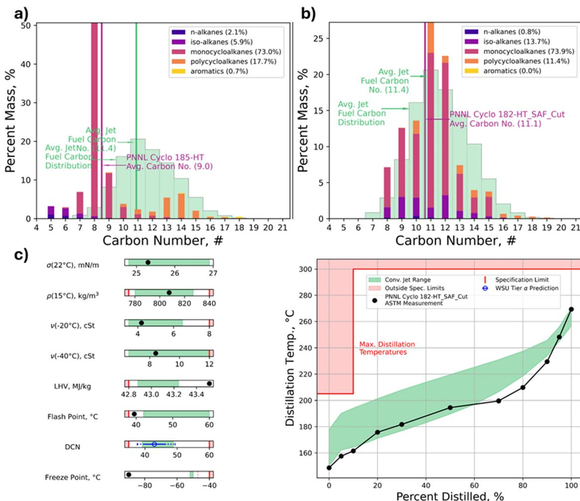
**Fig. 8** (a) Full distillate sample of the alkylated product after hydrotreatment (see Fig. S6d). (b) Jet range (>130 °C b.p. cut) after distillation. The green shaded region represents the carbon distribution of an average conventional jet fuel for reference. (c) Tier beta property measurement for the jet range hydrocarbons.
