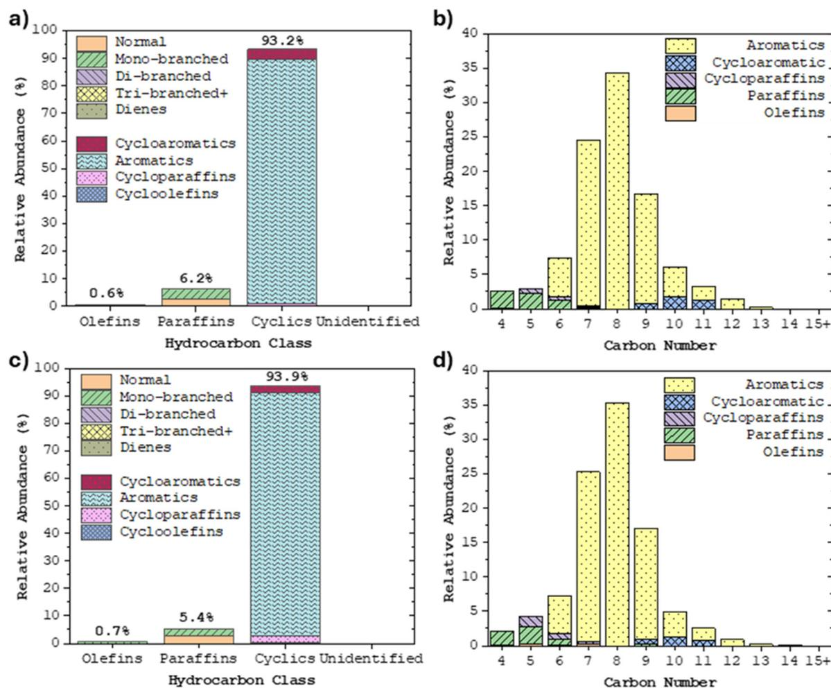
Fig. 4 Conversion of 1-butene over hydrothermally treated 1.5% Zn/ZSM-5 ( $\text{SiO}_2/\text{Al}_2\text{O}_3 = 23$ ) and resulting (a and c) liquid product classification and (b and d) carbon number distribution at (a and b) 8 and (c and d) 29 hours' time-on-stream ( $T = 515\text{ }^\circ\text{C}$ ,  $P = 75\text{ psig}$ ,  $\text{WHSV}_{1\text{-butene}} = 2.8\text{ h}^{-1}$ ).
