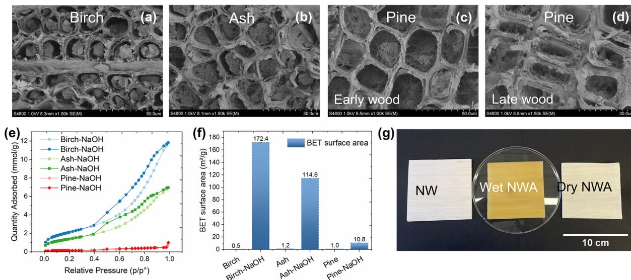
**Fig. 7** Universality and scalability of the approach. SEM images on the cross-section of (a) NaOH-treated birch, (b) NaOH-treated ash, (c) NaOH-treated pine on early wood region and (d) late wood region. (e) isotherm adsorption and desorption curves, (f) BET surface of different wood species after 24 h NaOH treatment, (g) photography of wet and dry NWA at large scale.
