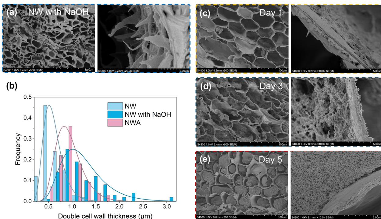
**Fig. 6** (a) Cross-section and cell wall morphology of NW right after NaOH treatment, SEM images showing substance separated from the cell wall, (b) double cell wall thickness histogram of NW, NW with NaOH and NWA, (c)–(e) SEM images showing the morphology evolution during aerogel formation, including partial liberation of cell wall materials to gradual filling of lumen with fibril networks.
