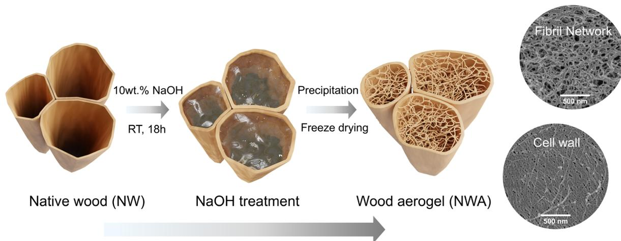
**Fig. 1** Schematic illustration of wood aerogel preparation. From cell wall swelling to the building of microfibril networks in lumen were shown. SEM images on the right display the fibril networks and porous cell wall of NWA.
