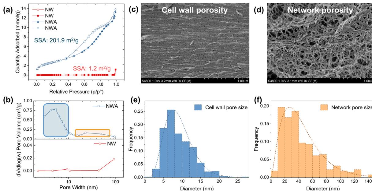
**Fig. 4** Mesoporous structure characterization of wood aerogels. (a) Isotherm adsorption and desorption curves and BET specific surface area of NW and NWA, (b) pore size distribution of NW and NWA. SEM images showing (c) cell wall porosity and (d) network porosity in NWA, corresponding diameter histogram of pores (e) in the cell wall, and (f) among fibril networks.
