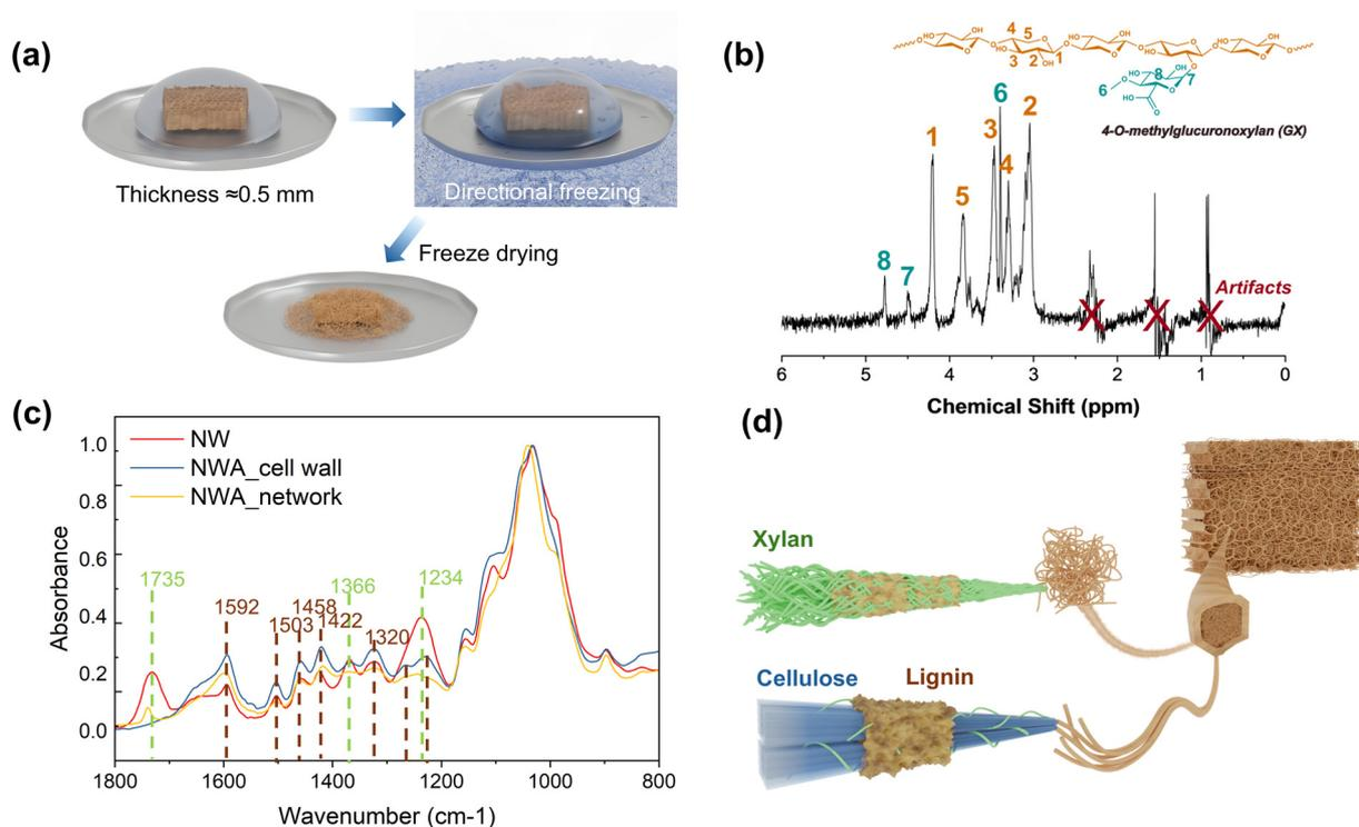
**Fig. 5** (a) Schematic diagram of utilizing directional freezing to isolate fibril networks from NWA, (b) diffusion-edited  $^1\text{H}$  NMR spectra of separated networks, (c) FTIR spectrum of NW, cell wall and networks of NWA, (d) schematic showing the composition of cell wall and network fibrils of NWA (blue crystals represent cellulose, green fibrils indicate xylan/hemicellulose and brown clusters represent lignin).
