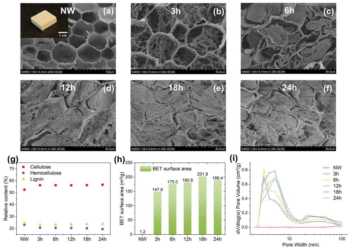
Fig. 2 (a) Photograph and SEM image of NW, (b)–(f) SEM images of wood samples *via* treatment time of 3 h, 6 h, 12 h, 18 h, 24 h, (g) relative content of cellulose, hemicellulose and lignin, (h) BET specific surface area and (i) pore size distribution of samples *via* different treatment time.
