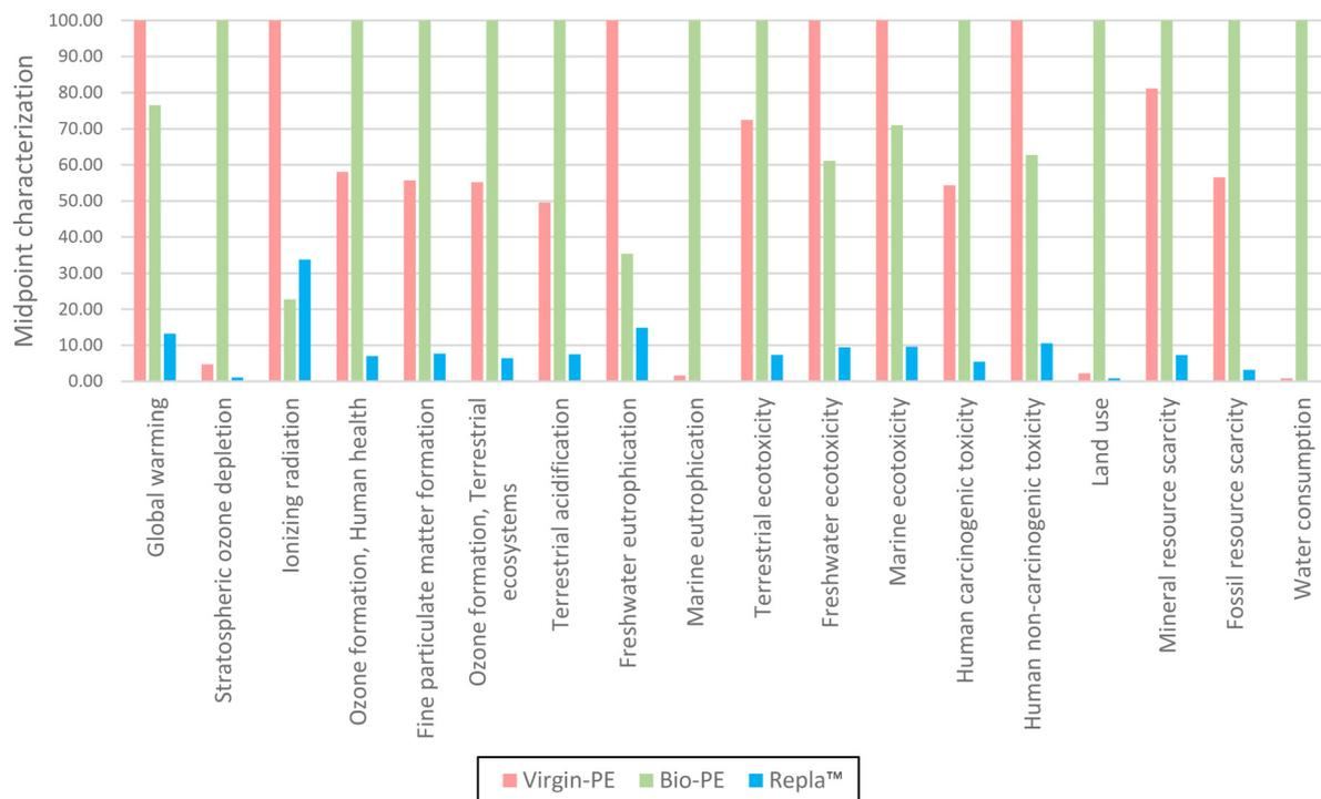
Fig. 3 Midpoint characterization comparisons of plastic pellets.
