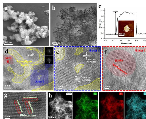
**Fig. 2** Physical characterization of CoOx/CoP-L: (a) SEM image, (b) TEM image, (c) thickness measurement diagram (inset: the atomic force microscope image), (d–f) HRTEM images (the illustration inside Fig. 1d is the selected area electron diffraction image), (g) ACTEM image and (h) TEM mapping images.
