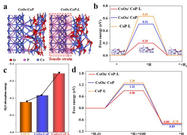
**Fig. 1** (a) Theoretical models of CoOx/CoP and CoOx/CoP-L, (b) calculated free energy diagrams of the acid HER pathway, (c) water adsorption energy diagram, and (d) calculated free energy diagrams of the alkaline HER pathway.
