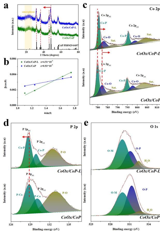
**Fig. 3** (a) XRD patterns of CoOx/CoP and CoOx/CoP-L, (b) the tensile strain coefficient diagram obtained by XRD fitting, (c–e) XPS spectra of CoOx/CoP and CoOx/CoP-L.
