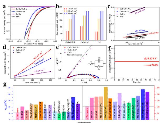
**Fig. 4** HER electrocatalytic properties of CoOx/CoP, CoOx/CoP-L, CoOx precursor and Pt/C in 1.0 M KOH: (a) LSV curves, (b) comparison diagram of voltage at current densities of 10, 100, and 200 mA cm<sup>-2</sup>, (c) Tafel slopes, (d) *C*<sub>dl</sub> curves, (e) Nyquist plots at a specific voltage of -0.15 V, (f) chronoamperometry test of CoOx/CoP-L and (g) comparison diagram of recently reported Co-based electrocatalysts.
