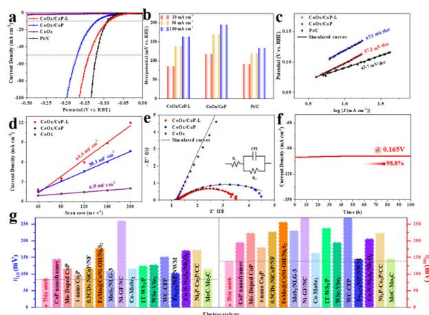
**Fig. 5** HER electrocatalytic properties of CoOx/CoP, CoOx/CoP-L, CoOx precursor and Pt/C in 0.5 M H<sub>2</sub>SO<sub>4</sub>: (a) LSV curves, (b) comparison diagram of voltage at current densities of 10, 50, and 100 mA cm<sup>-2</sup>, (c) Tafel slopes, (d) C<sub>dl</sub> curves, (e) Nyquist plots at a specific voltage of -0.15 V, (f) chronoamperometry test of CoOx/CoP-L and (g) comparison diagram of recently reported non-noble-metal-based electrocatalysts.
