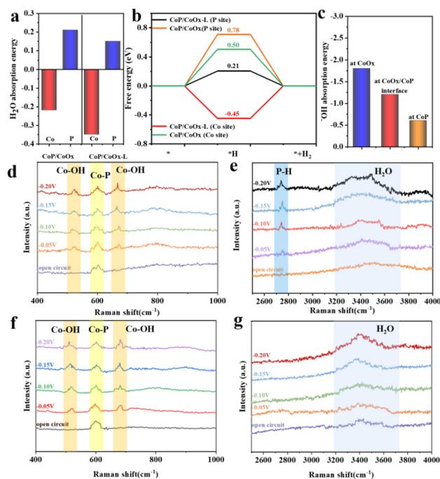
**Fig. 6** (a) H<sub>2</sub>O absorption capacity of site at CoOx/CoP and CoOx/CoP-L, (b) calculated free energy diagrams of H\*, (c) OH<sup>-</sup> absorption capacity of Co site at different positions in the CoOx/CoP-L model; *in situ* Raman spectra of (d and e) CoOx/CoP-L and (f and g) CoOx/CoP in the alkaline HER process.
