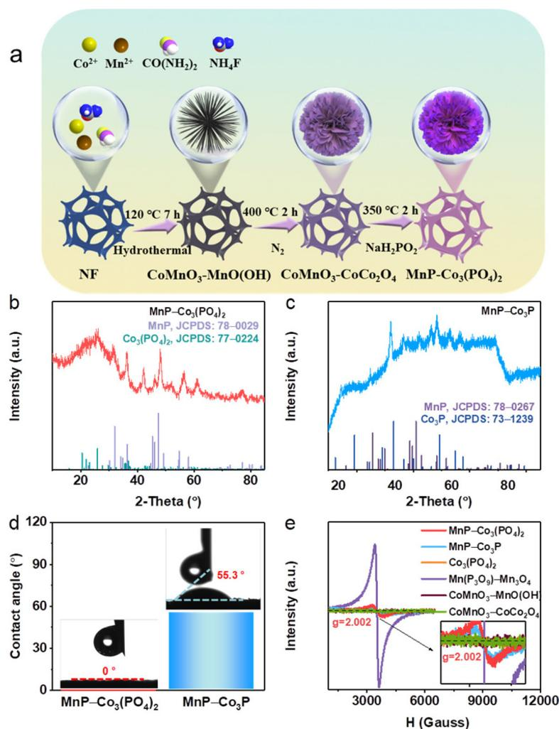
**Fig. 1** (a) Schematic illustration of the synthesis of  $\text{MnP-Co}_3(\text{PO}_4)_2/\text{NF}$ . XRD patterns of (b)  $\text{MnP-Co}_3(\text{PO}_4)_2/\text{NF}$  and (c)  $\text{MnP-Co}_3\text{P}/\text{NF}$ . (d) The contact angle test for  $\text{MnP-Co}_3(\text{PO}_4)_2/\text{NF}$  and  $\text{MnP-Co}_3\text{P}/\text{NF}$ . (e) Electron paramagnetic resonance (EPR) spectra of the different catalysts.
