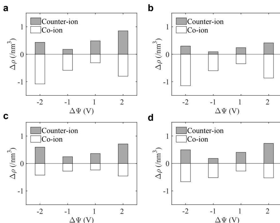
**Figure 4. Voltage-induced changes in ion population inside MXene pores. (a-d)** Change in the equilibrium pore ion population,  $\Delta\rho = \rho(\Delta\psi) - \rho(0V)$ , in pore with the widths of 0.7 nm **(a)**, 0.8 nm **(b)**, 1.0 nm **(c)**, and 1.2 nm **(d)**. The negative values indicate a decrease in the number of ions inside the pore.
