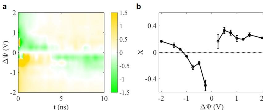
Fig. 5 Charging mechanism parameter  $X$  in a 1.0 nm MXene pore. (a) Time evolution of the voltage-dependent charging parameter  $X(\Delta\Psi, t)$  after a potential step, illustrating the relaxation toward equilibrium. The color scale denotes  $X(\Delta\Psi, t)$  resolved over an applied voltage  $\Delta\Psi$ , after time  $t$ . (b) Equilibrium values of  $X$  at different applied voltages, showing a clear asymmetry in charging response with applied voltage.
