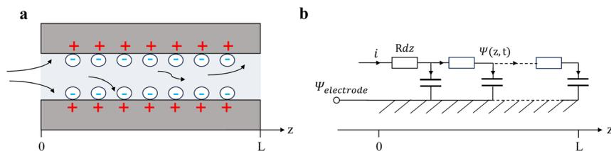
Fig. 2 Schematic of the transmission-line model. (a) Schematic of the charging process within a typical nanopore. (b) Corresponding equivalent circuit in the transmission-line model.  $R$  and  $C$  are the resistance and the capacitance 'per unit length' inside the electrodes, respectively.
