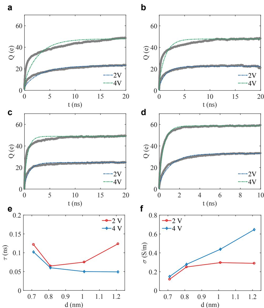
**Figure 6. Charging process at the nanoscale. (a-d)** Evolution of the total charge ( $Q$ ) on layered  $\text{Ti}_3\text{C}_2\text{O}_2$  electrodes of supercapacitors with  $[\text{Emim}][\text{BF}_4]$  dependent on the
