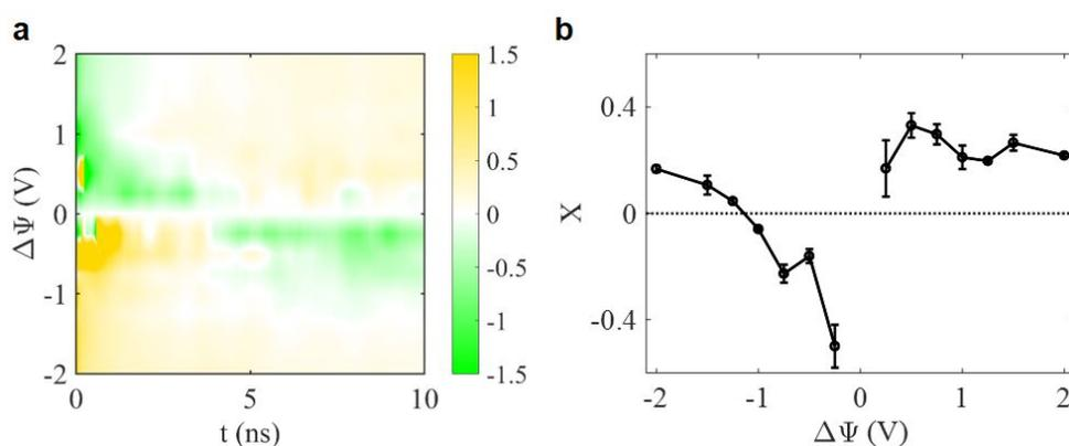
**Figure 5. Charging mechanism parameter  $X$  in 1.0 nm MXene pore. (a)** Time Evolution of the voltage-dependent charging parameter  $X(\Delta\Psi, t)$  after a potential step, illustrating the relaxation toward equilibrium. The color scale denotes  $X(\Delta\Psi, t)$  resolved over an applied voltage  $\Delta\Psi$ , after time  $t$ . **(b)** Equilibrium values of  $X$  at different applied voltages, showing a clear asymmetry in charging response with applied voltage.
