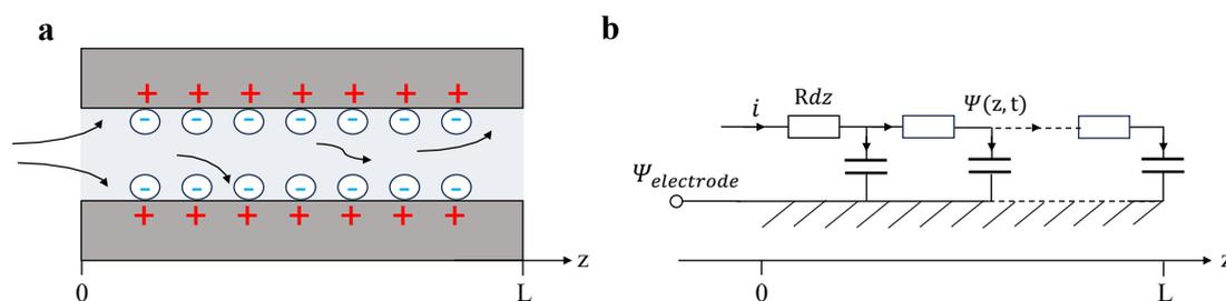
**Figure 2. Schematic of the Transmission Line Model.** (a) Schematic of the charging process within a typical nanopore. (b) Corresponding equivalent circuit in the transmission line model.  $R$  and  $C$  are the resistance and the capacitance ‘per unit length’ inside the electrodes, respectively.
