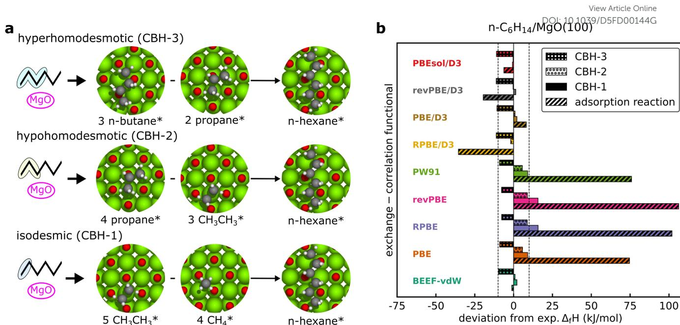
**Figure 4** a) CBH reaction scheme for n-hexane adsorbed on MgO(100) and b) deviation of the n-C<sub>6</sub>H<sub>14</sub>\* enthalpies of formation derived via the CBH scheme and adsorption reaction from the experimental value. The colored area in the Lewis structure indicates the conserved fragments at the different CBH rungs.
