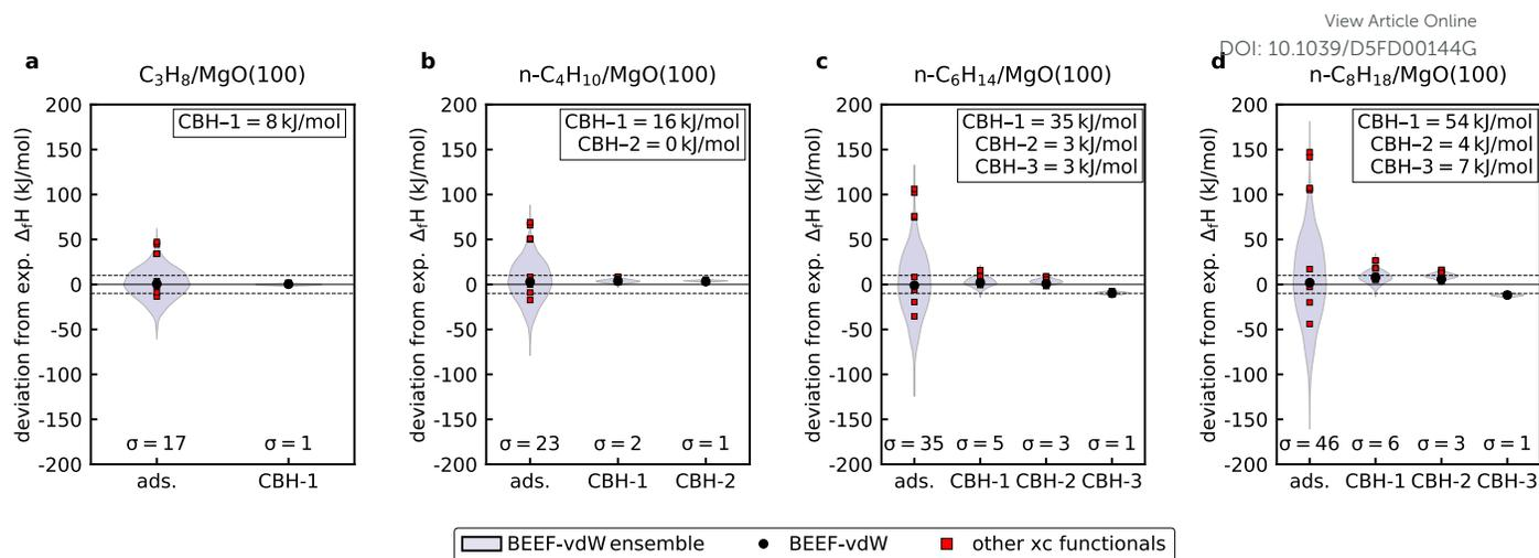
**Figure 5** Benchmarking of the adsorption reaction and CBH method for physisorbed a)  $C_3H_8^*$ , b)  $n-C_4H_{10}^*$ , c)  $n-C_6H_{14}^*$ , and d)  $n-C_8H_{18}^*$  on  $MgO(100)$ . Only CBH-1 is possible for  $C_3H_8^*$  and CBH-2 is the highest rung for  $n-C_4H_{10}^*$ , whereas CBH-3 can be used for  $n$ -hexane and  $n$ -octane. The contour shows the uncertainty spanned by the BEEF ensemble.
