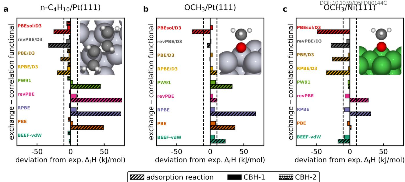
**Figure 2** Comparison of computed and experimental enthalpies of formation of a)  $n\text{-C}_4\text{H}_{10}^*$  on Pt(111), b)  $^*\text{OCH}_3$  on Pt(111), and c)  $^*\text{OCH}_3$  on Ni(111) using the conventional adsorption reaction approach and the error cancellation reactions of the connectivity-based hierarchy. Experimental enthalpies of adsorption are reported in Table 2 and the dashed lines represent the experimental accuracy of  $\pm 10 \text{ kJ mol}^{-1}$ .
