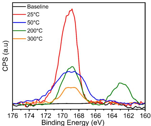
Fig. 6 S2p XPS spectra of Pt NCs before (black spectrum) and after their exposure  $\text{H}_2\text{SO}_4$ . XPS measurements of the poisoned NCs were acquired at room temperature (red spectrum), and after annealing at 50 °C (blue spectrum), 200 °C (green spectrum) and 300 °C (orange spectrum).
