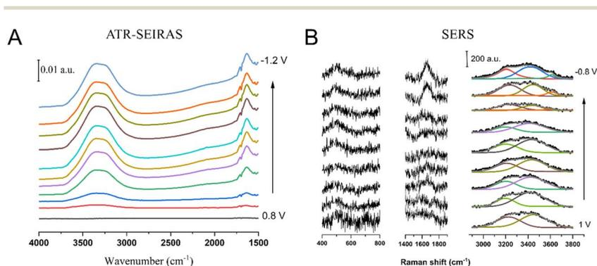
Fig. 2 (A) ATR-SEIRAS and (B) SER spectra of the Au-electrolyte interface in 1 M KOH solution (100%  $\text{H}_2\text{O}$ ) within the potential regions between 0.8 and  $-1.2$  V (A) and between 1 and  $-0.8$  V (B). The differential spectra in (A) used the spectrum at 0.8 V as background.
