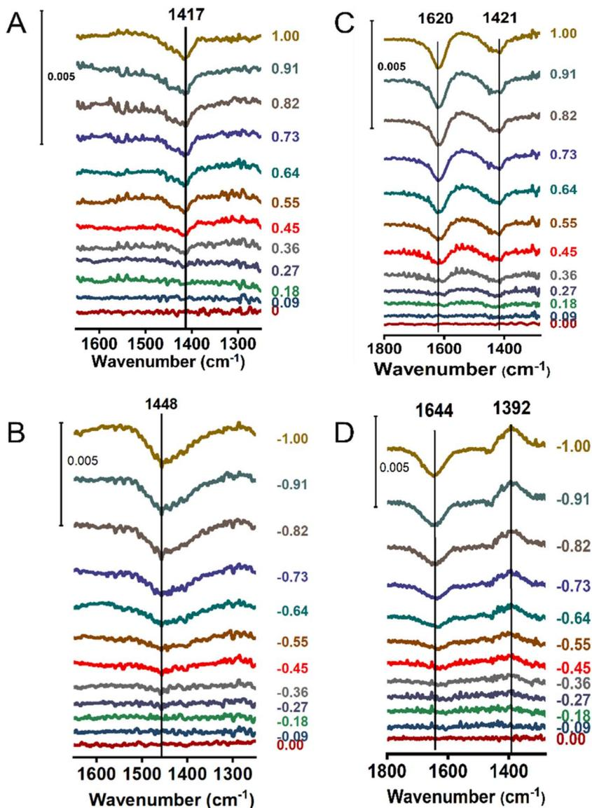
Fig. 6 The bending band region of 1 : 3 H<sub>2</sub>O : D<sub>2</sub>O in (A) the dl region and (B) HER region. The bending band region of 3 : 1 H<sub>2</sub>O : D<sub>2</sub>O in the (C) dl region and (D) HER region.
