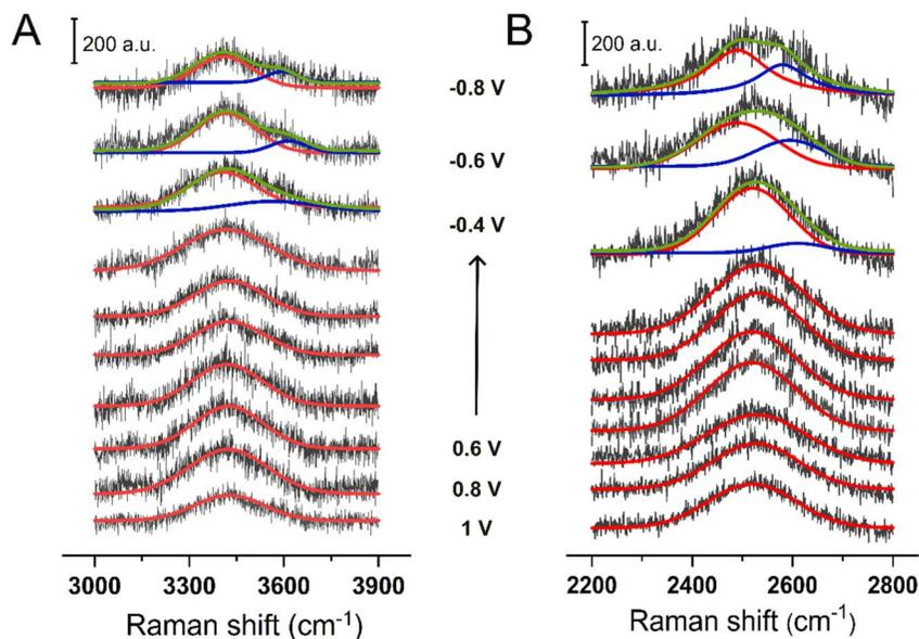
Fig. 7 The changes in (A)  $\nu_{\text{OH}}$  band in 1 : 3  $\text{H}_2\text{O}:\text{D}_2\text{O}$  solution and (B)  $\nu_{\text{OD}}$  band of H–O–D 3 : 1  $\text{H}_2\text{O}:\text{D}_2\text{O}$  with applied bias.
