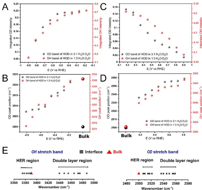
Fig. 5 The change in the integrated band intensity and the peak position of the HER region (A and B) and dl region (C and D). (E) The range of wavenumbers of the  $\nu_{\text{OH}}$  and  $\nu_{\text{OD}}$  bands in the dl and HER region as compared to the bulk solution.
