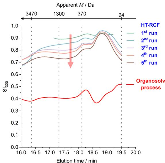
Fig. 8  $SI_{320}(M)$  profiles of HT-RCF lignin oils from post-consumer cardboard obtained over five consecutive HT-RCF runs with RANEY<sup>®</sup> Ni (2-propanol/H<sub>2</sub>O, 7 : 3 v/v; 200 °C; 3 h; H<sub>2</sub>-free), compared with the  $SI_{320}(M)$  profile of organosolv lignin.
