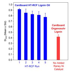
Fig. 9 Evolution of  $SI_{320}$  with catalyst recycle and linear deactivation model. A linear fit to  $SI_{320}$  vs. run count gives:  $SI_{320} = (0.951 \pm 0.007) - (0.03652 \pm 0.00371) \times n$  ( $r^2 = 0.95$ ), where "n" is the run number. Extrapolation to the mean value for organosolv lignin indicates convergence at approximately the 15th run, around 45 hours of HT-RCF operation.
