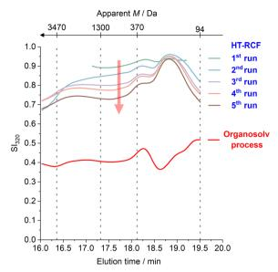
Fig. 8 SI<sub>320</sub>(M) profiles of HT-RCF lignin oils from post-consumer cardboard obtained over five consecutive HT-RCF runs with RANEY® Ni (2-propanol/H2O, 7:3 v/v; 200 °C; 3 h;  $H_2$ -free), compared with the  $SI_{320}(M)$  profile of organosoly lignin.
