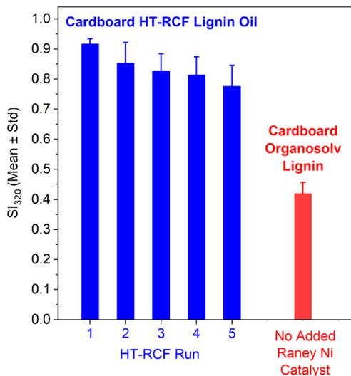
Fig. 9 Evolution of  $SI_{320}$  with catalyst recycle and linear deactivation model. A linear fit to  $SI_{320}$  vs. run count gives:  $SI_{320} = (0.951 \pm 0.007) - (0.03652 \pm 0.00371) \times n$  ( $r^2 = 0.95$ ), where “ $n$ ” is the run number. Extrapolation to the mean value for organosolv lignin indicates convergence at approximately the 15th run, around 45 hours of HT-RCF operation.
