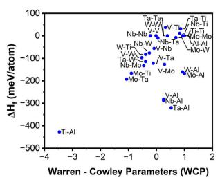
Fig. 3 The formation enthalpy of binary ground-state and ordered compounds from the literature<sup>56</sup> versus the Warren–Cowley parameters (WCP) from the 1NN shell of corresponding element pairs.
