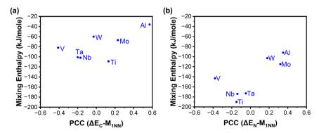
Fig. 6 Metal—C or metal—N enthalpy of mixing values from the literature<sup>57</sup> plotted against: (a) the Pearson correlation coefficient (PCC) between the carbon doping energy,  $\Delta E_{\rm C}$ , and the number of metal atoms in the 1NN shell of the dopant (M<sub>1NN</sub>); and (b) the PCC between the nitrogen doping energy,  $\Delta E_{\rm N}$ , and M<sub>1NN</sub>.
