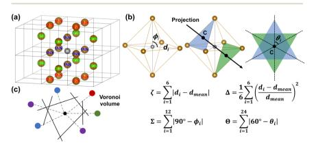
Fig. 1 (a) The illustration of the first-, second-, and third-nearest-neighbor (1NN, 2NN, and 3NN) shells surrounding an octahedral site in a body-centered-cubic (BCC) lattice. (b) The illustration and definition of OctaDist parameters<sup>25</sup>  $\zeta$ ,  $\Delta$ ,  $\Sigma$ , and  $\Theta$ , which describe the distance, tilting, angle, and torsional distortion; and (c) the illustration of the Voronoi volume.
