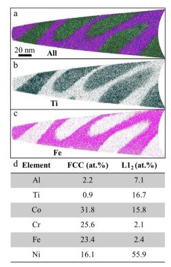
Fig. 5 APT results from the 90CRA condition. (a) A 2D section of the superimposition of all raw ion maps (Al = blue, Ti = dark green, Co = blue, Cr = light pink, Fe = dark pink, Ni = green), (b) Ti raw ion map section, (c) Fe raw ion map section, and (d) FCC and  $L1_2$  compositions in the 90CRA condition.
