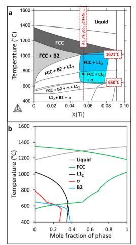
Fig. 1 (a) Pseudo-binary isopleth for  $Al_{0.5-x}Ti_xCo_{1.5}CrFeNi_{1.5}$  (x=0 to 0.5 in relative mole fraction). (b) Phase fraction vs. temperature diagram for  $Al_{0.2}Ti_{0.3}Co_{1.5}CrFeNi_{1.5}$ .
