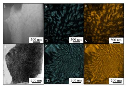
Fig. 4 (a) HAADF-STEM image and (b) Ti and (c) Ni STEM-EDS maps from a non-recrystallized grain in the 60CRA condition show blocky  $L1_2$  precipitation. (d) HAADF-STEM image and (e) Ti and (f) Ni STEM-EDS maps from a recrystallized grain in the 90CRA condition show rod-like  $L1_2$  precipitation.
