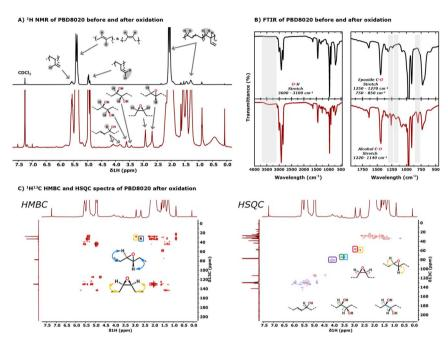
Fig. 3 (A) <sup>1</sup>H NMR spectra of unfunctionalised PBD8020 (black trace) and oxyfunctionalised PBD8020 (red trace). (B) FTIR spectra of unfunctionalised PBD8020 (black trace) and oxyfunctionalised PBD8020 (red trace). (C) <sup>1</sup>H<sup>13</sup>C HMBC and HSQC spectra of oxyfunctionalised PBD8020.
