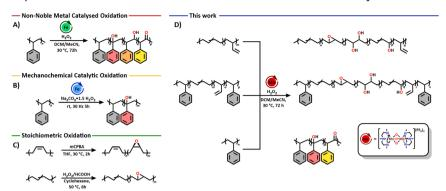
Scheme 1 (A) Non-noble metal catalysed oxidation of polystyrene. (B) Solvent-free mechanochemical catalytic oxidation of polystyrene. (C) Stoichiometric oxidation of polybutadiene by mCPBA and  $H_2O_2$ /formic acid. (D) This work on the oxidation of polystyrene and polybutadiene using a robust manganese oxidation catalyst.
