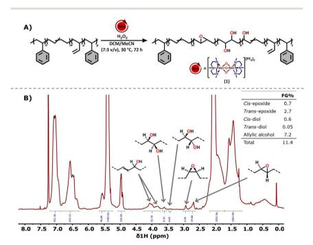
Fig. 4 (A) Catalytic oxyfunctionalisation conditions tested on SBS using the tri-oxo (1) bridged analogue of MnTACN. (B) <sup>1</sup>H NMR spectrum after the oxyfunctionalisation of styrene-butadiene-styrene (SBS) block-co-polymer, with the corresponding FG% of each installed oxyfunctional group.
