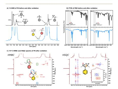
Fig. 2 (A) <sup>1</sup>H NMR spectra of unfunctionalised PS (black trace) and oxyfunctionalised PS (blue trace). (B) FTIR spectra of unfunctionalised PS (black trace) and oxyfunctionalised PS (blue trace). (C) <sup>1</sup>H<sup>13</sup>C HMBC and HSQC spectra of oxyfunctionalised polystyrene.
