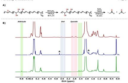
Fig. 5 (A) Ring-opening of the epoxides installed on the PBD backbone using sulfuric acid and subsequent oxidative cleavage of the diol-moieties. (B)  $^1$ H NMR spectra of oxyfunctionalised PBD8020 (red trace), fully alcohol functionalised PBD8020 after ring opening of the epoxides (blue trace) and oxidatively cleaved PBD8020 to di-aldehydes (green trace). The  $\Delta$  in the blue trace is residual THF.
