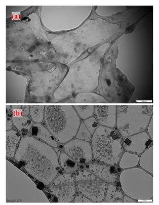
Fig. 6 TEM micrographs of FeCoNiCuPt HEA nanoparticles showing residual NaCl particles when capped with (a) oleylamine and (b) hexadecylamine introduced prior to washing (*in situ* capping) out the NaCl particles.
