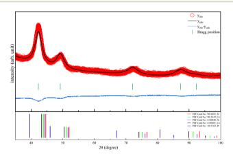
Fig. 1 The Rietveld-refined XRD patterns of the uncapped FeCoNiCuPt sample and corresponding PDF standard patterns of constituent elements of the  $Fm\overline{3}m$  (225) space group. Red circles, black line, blue line and green vertical signs represent the observed  $(y_{\text{obs}})$ , calculated  $(y_{\text{calc}})$ , the difference between the observed and calculated spectra  $(y_{\text{obs}} - y_{\text{calc}})$ , and Bragg positions, respectively.
