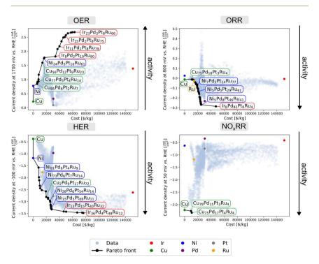
Fig. 8 Pareto fronts for the electrochemical activity of the four reactions vs. the cost of the catalysts.<sup>27</sup> Single element samples are marked in different colours. Representative quaternary compositions along the Pareto front are indicated.
