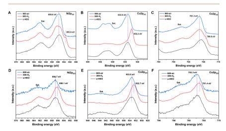
Fig. 4 XPS spectra for pristine, reduced (5%  $H_2$ /Ar at 600 °C), and re-oxidized (air at 900 °C) c-HEO (A: Ni 2p region; B: Cu 2p region; C: Co 2p region), and pristine, reduced (5%  $H_2$ /Ar at 300 °C), and re-oxidized (air at 600 °C) a-HEO (D: Ni 2p region; E: Cu 2p region; F: Co 2p region) samples.
