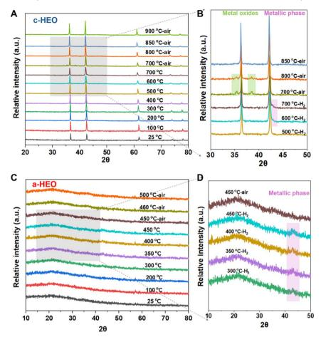
Fig. 2 In situ XRD patterns of c-HEO (A and B) and a-HEO (C and D) collected at programmed temperatures under reducing (2% H<sub>2</sub> in He) and oxidative (air) atmospheres.
