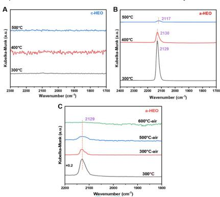
Fig. 7 CO-DRIFTS results of c-HEO (A) and a-HEO (B) at different reduction temperatures under 5%  $\rm H_2/Ar$  atmosphere and a-HEO (C) at different oxidation temperatures under air atmosphere.
