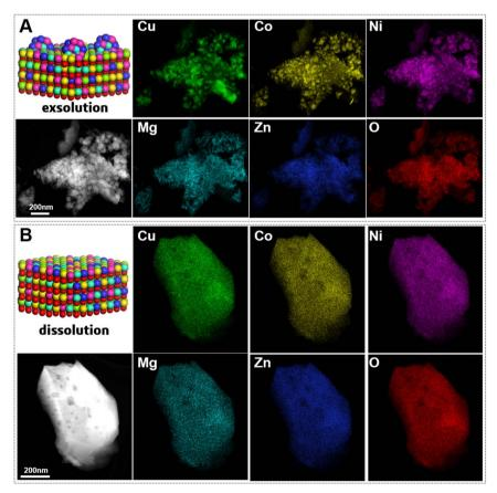
Fig. 5 Microscopy of treated samples of c-HEO after reduction under 5% H<sub>2</sub> at 600 °C (A) and subsequent oxidation under air at 900 °C (B).
