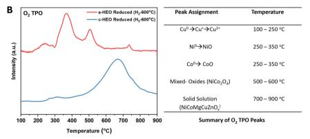
Fig. 3 (A)  $\rm H_2$  TPR analysis of a-HEO and c-HEO with summary of  $\rm H_2$  TPR peaks; (B)  $\rm O_2$  TPO analysis of a-HEO reduced at 600 °C in  $\rm H_2$  and c-HEO reduced at 600 °C with summary of  $\rm O_2$  TPO peaks.
