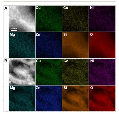
Fig. 6 Microscopy of treated samples of a-HEO after reduction under 5% H<sub>2</sub> at 300 °C (A) and subsequent oxidation under air at 350 °C (B).
