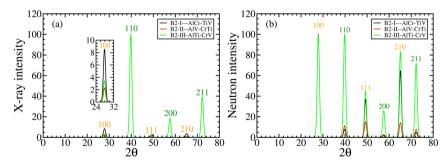
Fig. 3 X-ray (a) and neutron (b) diffraction patterns of B2 variants. Miller indexing is based on the 2-atom cubic cell of lattice constant 3.2 Å. Miller indices corresponding to a BCC lattice (A2) are colored in dark green; B2 (CsCl) peak indices are orange. Cu-K $\alpha$  radiation ( $\lambda=1.5406$  Å) is assumed for X-rays, and the same wavelength is chosen for the neutron pattern.
