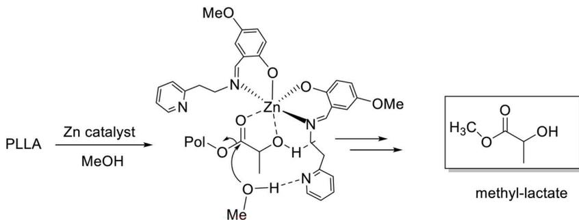
Scheme 2 Solvent-free methanolysis of PLA by complex 1.
