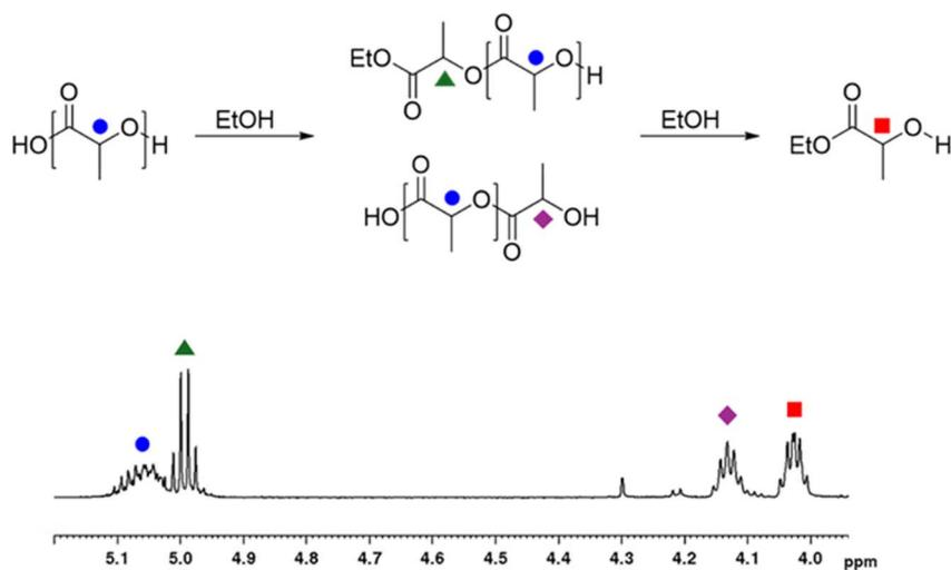
Fig. 2 <sup>1</sup>H NMR spectrum (600 MHz, CDCl<sub>3</sub>, 298 K) with methine group assignments for a PLLA ethanolysis.
