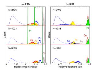
Fig. 8 Distributions of maximum fragment size predicted for 2406-, 4033-, and 6266atom nanoparticles at equicomposition using the (a) EAM or (b) SMA potentials, normalized by the total nanoparticle size. The dashed lines are the result expected for the corresponding ideal solid solutions.
