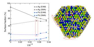
Fig. 7 Surface fractions in silver and palladium predicted for N-atom nanoparticles at equicomposition, as a function of their inverse radius  $1/N^{1/3}$ , predicted by the EAM and SMA potentials, and extrapolation to the (111) slab for  $N^{-1/3} \rightarrow 0$ . A typical configuration for the largest nanoparticle described by the SMA potential is shown in the right panel, emphasizing the surface desorption in silver with the red ellipses.
