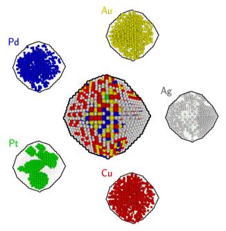
Fig. 5 Elemental distribution in a low-energy configuration of the 4033-atom nanoparticle at equicomposition, as predicted using the EAM potential.
