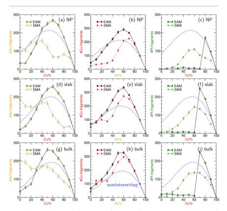
Fig. 4 Average number of disconnected fragments of a given element, as the overall concentration of another element is increased in 4033-atom nanoparticles (upper panels), 4032-atom (111) slabs (middle panels), or 4000-atom FCC periodic samples (lower panels), predicted from the EAM and SMA potentials. The dashed blue line is the expected result for the ideal solid solution. (a, d and g) Au vs. Cu; (b, e and h) Cu vs. Au; (c, f and i) Pt vs. Cu.
