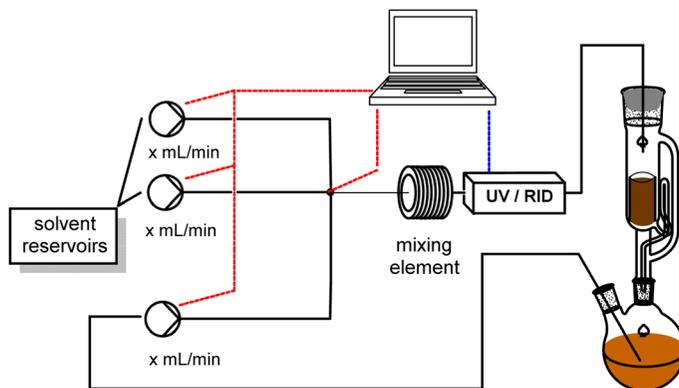
Fig. 2 Scheme of pump-enabled Soxhlet-extractions of technical lignins.
