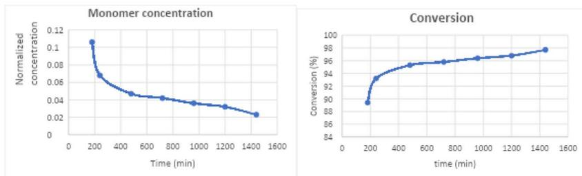
Fig. 4 Homopolymerization of P2VPPS in a continuous flow reactor set-up: flow  $0.2 \text{ ml min}^{-1}$  up to  $1 \text{ ml min}^{-1}$  using a step of  $0.1 \text{ ml min}^{-1}$  showed the correlation of monomer concentration and the conversion percentage in a quiescent experiment under ambient time and pressures.
