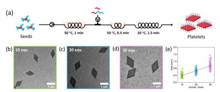
Fig. 5 Flow living CDSA preparing size-controllable platelets using PLLA $_{12}$ /PLLA $_{45}$ -b-PDMAEMA $_{183}$ : (a) scheme of preparing platelets in the flow reactor, (b), (c) and (d) are TEM images of platelets prepared at various unimer-to-seed ratios, and (e) linear fit of area upon different unimer-to-seed ratios. Scale bar = 1  $\mu$ m. Platelet size was analyzed from at least 100 particles.
