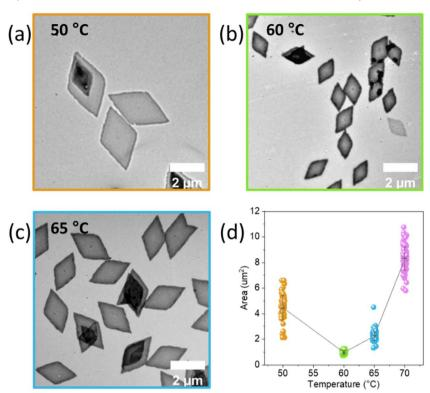
Fig. 2 Platelets prepared at different temperatures: (a), (b), and (c) are TEM images of platelets prepared at 50, 60, and 65 °C, and (d) area variation upon temperature. Scale bar  $= 2 \mu m$ . Platelet size was analyzed from at least 100 particles.
