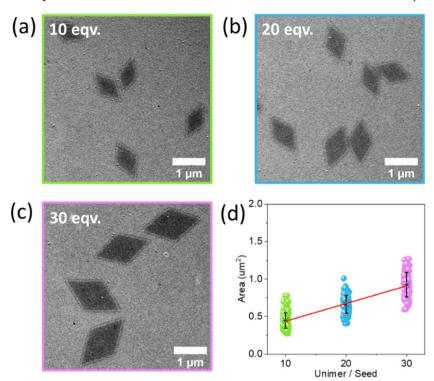
Fig. 4 Size-controllable platelets prepared by living CDSA using PLLA $_{12}$ /PLLA $_{45}$ -b-PDMAEMA $_{183}$  at mass ratio of 1/1: (a), (b), and (c) are TEM images of platelets prepared at various unimer-to-seed ratios, and (d) linear fit of area upon different unimer-to-seed ratios. Scale bar = 1  $\mu$ m. Platelet size was analyzed from at least 100 particles.
