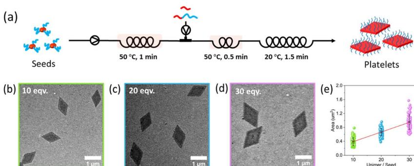
Fig. 5 Flow living CDSA preparing size-controllable platelets using PLLA<sub>12</sub>/PLLA<sub>45</sub>-*b*-PDMAEMA<sub>183</sub>: (a) scheme of preparing platelets in the flow reactor, (b), (c) and (d) are TEM images of platelets prepared at various unimer-to-seed ratios, and (e) linear fit of area upon different unimer-to-seed ratios. Scale bar = 1 μm. Platelet size was analyzed from at least 100 particles.
