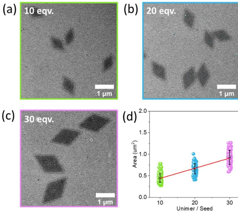
Fig. 4 Size-controllable platelets prepared by living CDSA using PLLA<sub>12</sub>/PLLA<sub>45</sub>-*b*-PDMAEMA<sub>183</sub> at mass ratio of 1/1: (a), (b), and (c) are TEM images of platelets prepared at various unimer-to-seed ratios, and (d) linear fit of area upon different unimer-to-seed ratios. Scale bar = 1 μm. Platelet size was analyzed from at least 100 particles.
