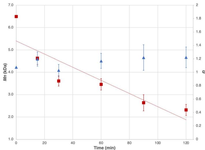
Fig. 10 Exemplar aliquot analysis of PCHC CDP reaction (Table 2, entry 4) by GPC showing linear decrease in  $M_n$  (red, squares) and variation in  $D$  (blue, triangles). Error bars are calculated from the Wyatt ASTRA Software report.
