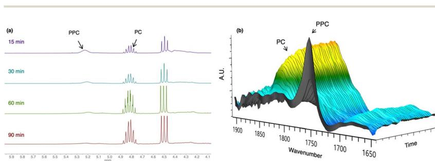
**Fig. 1** (a) Stacked <sup>1</sup>H NMR spectra of aliquots taken for Table 1, entry 1 showing the formation of PC over time and (b) 3D FT-IR spectrum showing the formation of the cyclic carbonate peak (~1816 cm<sup>-1</sup>) and disappearance of the polycarbonate peak (~1750 cm<sup>-1</sup>) for Table 1, entry 6.
