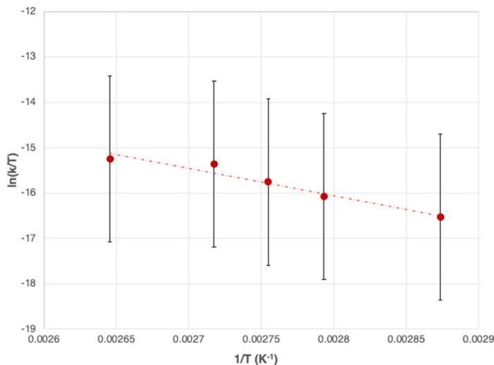
Fig. 7 Eyring plot of PPC CDP in toluene.  $y = -6034x + 0.84$ ,  $R^2 = 0.9496$ . Error analysis performed as reported by Lente *et al.*<sup>51</sup>
