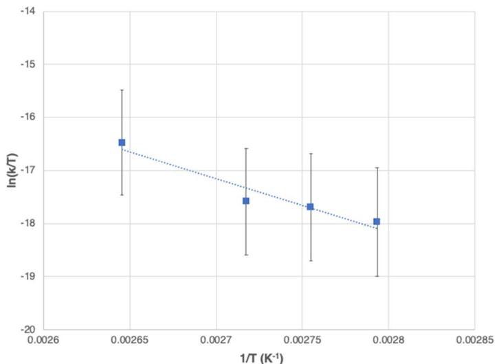
Fig. 9 Eyring plot of PCHC CDP in toluene.  $y = -10045.6x + 1.0$ ,  $R^2 = 0.9246$ . Error analysis performed as reported by Lente *et al.*<sup>51</sup>
