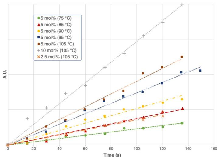
Fig. 6 Initial rates of cyclic carbonate formation taken from FTIR spectra around  $1816\text{ cm}^{-1}$ .  $k_{\text{app}}$  values listed in Table 4 are taken from the slopes of the linear trendlines.  $R^2$  values for all trends are  $>0.99$ .
