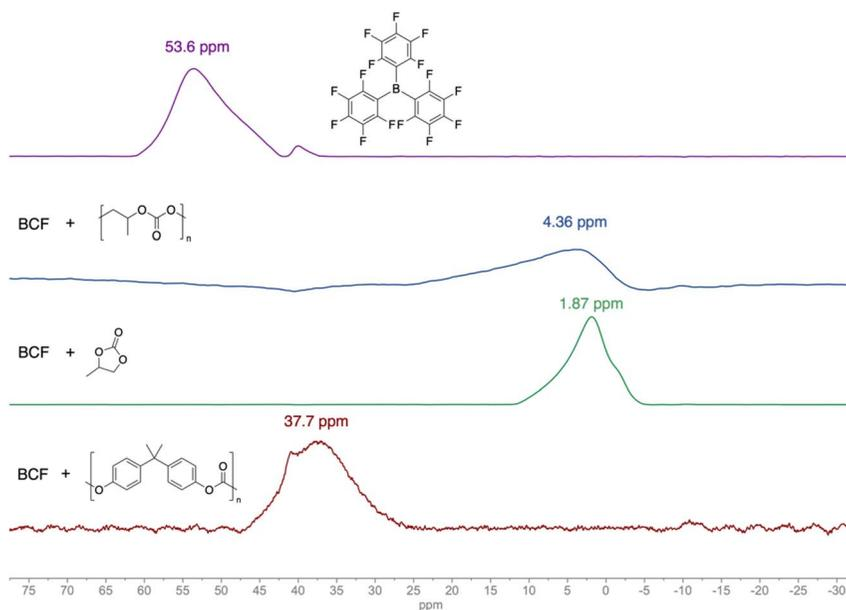
Fig. 3 <sup>11</sup>B NMR spectra (160 MHz, CDCl<sub>3</sub>) of BCF alone (top, purple) and in the presence of PPC (second, blue), PC (third, green), or PBPAC (bottom, red).
