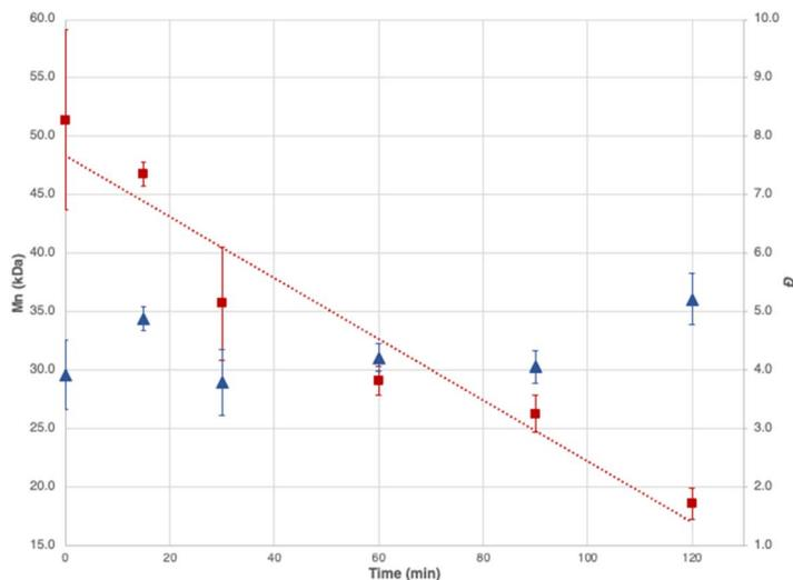
Fig. 5 Aliquot analysis by GPC of PPC (Table 1, entry 4) showing a linear decrease in  $M_n$  (red, squares) and minimal variation in  $D$  (blue, triangles). Error bars are calculated from the Wyatt ASTRA Software report.
