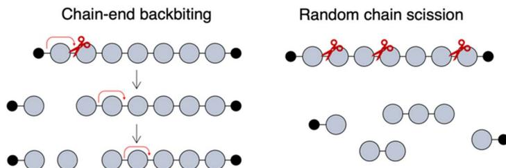
**Fig. 4** Schematic of two possible CDP pathways presented in this work.<sup>31,50</sup>
