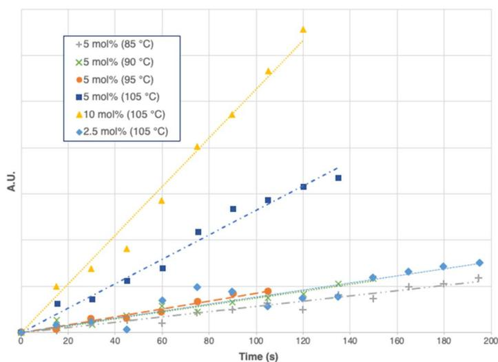
Fig. 8 Initial rates of cyclic carbonate formation during PCHC CDP taken from FTIR spectra at  $\sim 1816 \text{ cm}^{-1}$ .  $k_{\text{app}}$  values listed in Table 5 are taken from the slopes of the linear trendlines.  $R^2$  values for all trends are  $>0.95$ .
