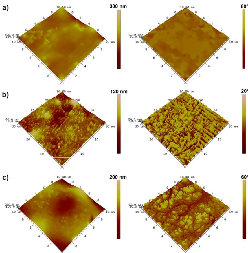
Fig. 4 Height (on the left) and phase contrast (on the right) tapping mode AFM micrographs of (a) **PM** homopolymer (sample from run 1 of Table 1), (b) **PME** copolymer (sample from run 5 of Table 1), and (c) **PMEI** copolymer (sample from run 9, Table 3).
