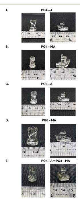
Fig. 4 SLA printing results of (A) PG4–A, (B) PG4–MA, (C) PG6–A, (D) PG6–MA and (E) PG4–A + PG4–MA, representing printed scaffolds, rook and boat, from each resin to test printability.
